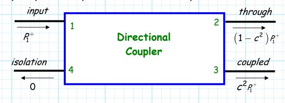
Note however, that any of the coupler ports can be an input, with a different through, coupled and isolation port for each case.
