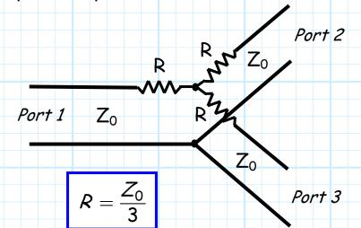
For this design, the ports are matched! However, the resistors make the device lossy:
