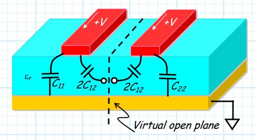
Note the  $2C_{12}$  capacitors have been "disconnected", and thus the capacitance per unit length of each transmission line, in the **even** mode, is thus:
