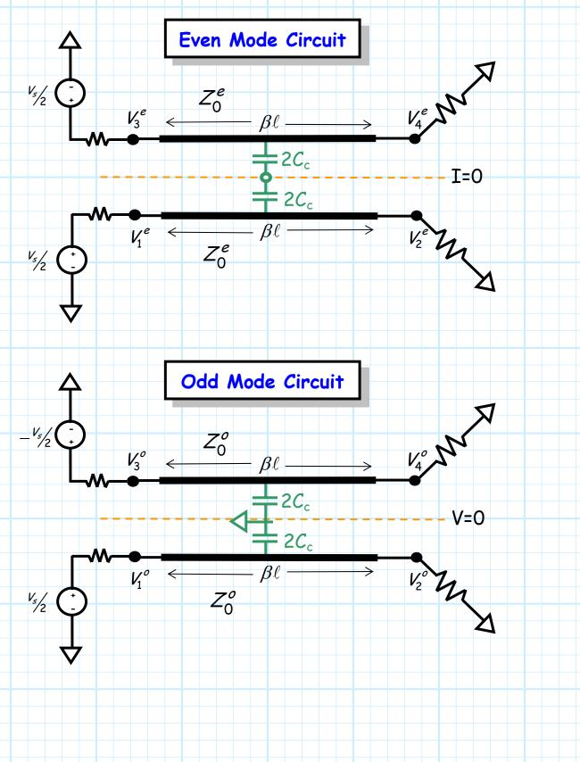
Note that the capacitive coupling associated with these modes are different, resulting in a different characteristic impedance of the lines for the two cases (i.e.,  $Z_0^e$ ,  $Z_0^o$ ).
