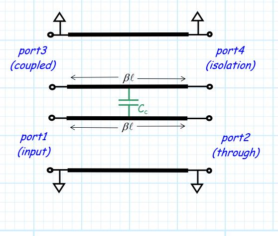
Q: But, how do we design a coupled-line coupler with a specific coupling coefficient c?
