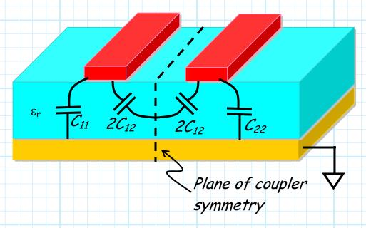
Note we have divided the  $C_{12}$  capacitor into **two series** capacitors, each with at value 2  $C_{12}$ .
