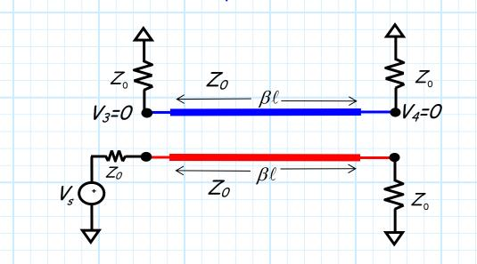
This makes sense! After all, if no coupling occurs, then the characteristic impedance of each line is unaltered by the presence of the other—their characteristic impedance is  $Z_0$ regardless of "mode".
