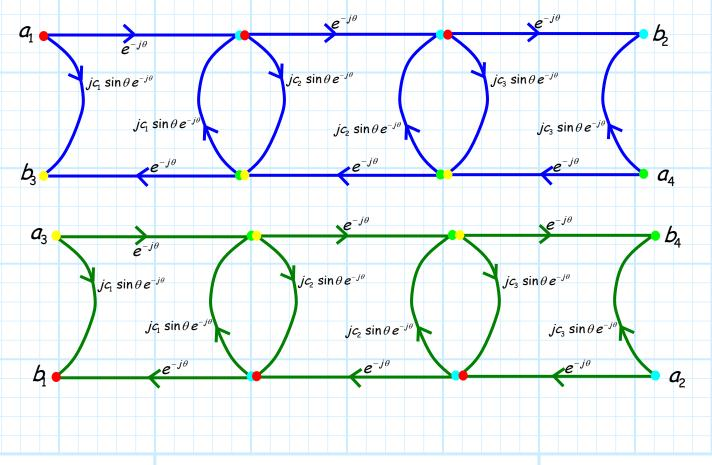
Note that these two graphs are essentially identical, and emphasize the symmetric structure of the coupled-line coupler.
