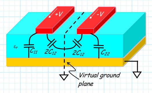
Thus, the capacitance per unit length of each transmission line, in the odd mode, is thus:
