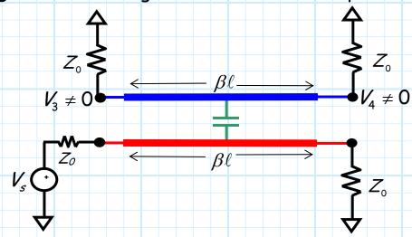
Now, our first step in performing the odd/even mode analysis will be to determine scattering parameter  $S_{11}$ . To accomplish this, we will need to determine voltage  $V_1$ :
