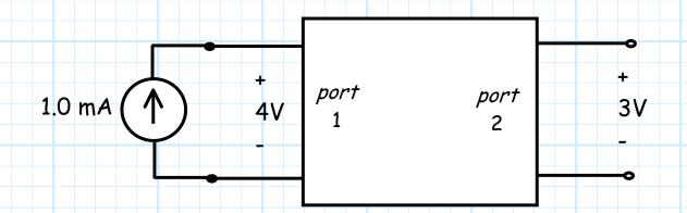
Determine both the impedance and admittance matrices of this device.
