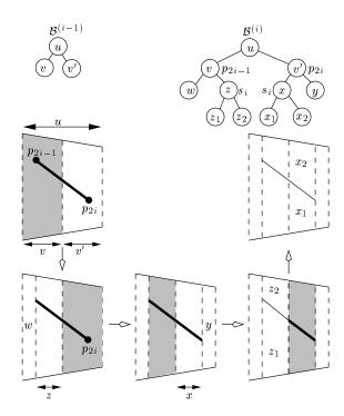
Figure 1: The BSP  $\mathcal{B}^{(i-1)}$ , the sequence of cuts made in the ith stage, and BSP  $\mathcal{B}^{(i)}$ . At each step, the shaded trapezoids are split. Portions of  $s_i$  that lie in the interior of a trapezoid are drawn using thick lines.
