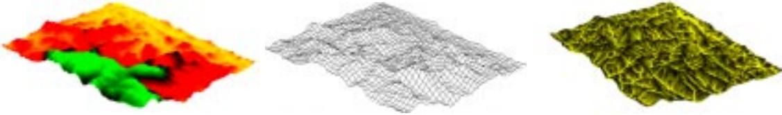
Figure 1: Terrain, its grid-based DEM, and a representation of its topographic convergence index.
