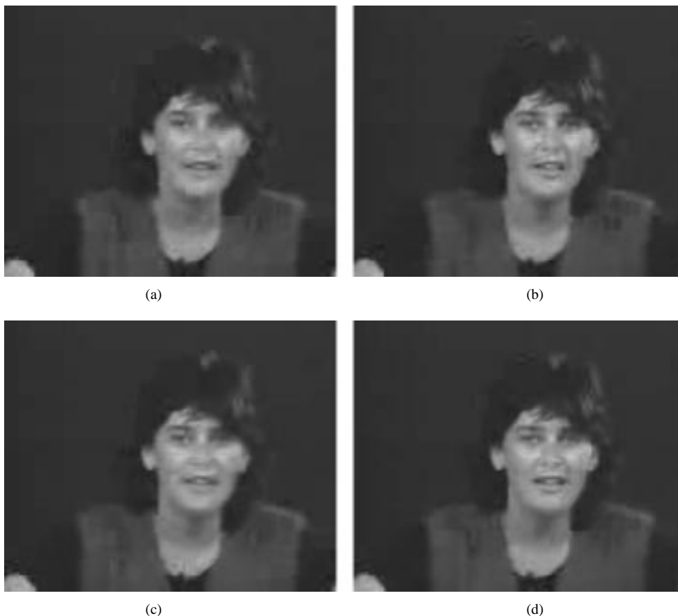
Fig. 10. Frame 27 of the Miss America sequence as encoded using the heuristic motion estimation algorithms. Only the luminance component is shown. (a) H1-A. (b) H2-A. (c) H1-WH. (d) H2-WH.
