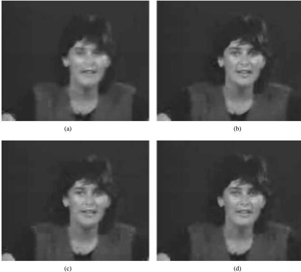
Fig. 9. Frame 27 of the Miss America sequence as encoded using the PVRG and explicit-minimization motion estimation algorithms. Only the luminance component is shown. (a) PVRG. (b) RD. (c) M1. (d) M2.
