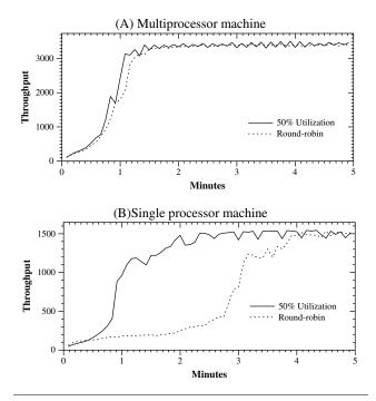
**Figure 2.** Websphere J2EE Application Server running Trade 6.1, performance of a round-robin scheduler compared to 50% utilization. The graphs show throughput over time, where higher is better. Rampup time of the round-robin scheduler is significantly degraded when CPU resources are constrained.
