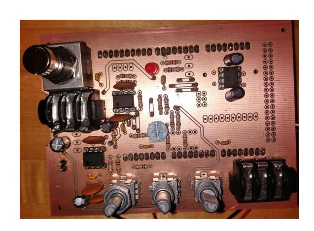
Signal from a guitar is amplified in a non-inverting/inverting op amp network, and sent to different ADCs on the Arduino. Potentiometers are used to adjust gain, and are referenced in the code for the modulation of volume and the effect depth. A footswitch is used to toggle on/off an effect. The original and processed signals generated at the DACs are read in parallel and added, for faster real time output of effects like delay. The output is amplified for connection to a guitar amp.
