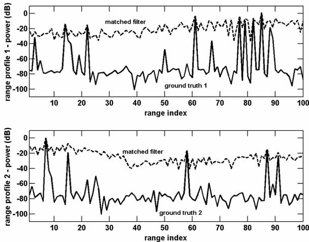
Fig. 4. Matched filter results for multistatic radar reception with spatial beamforming separation
