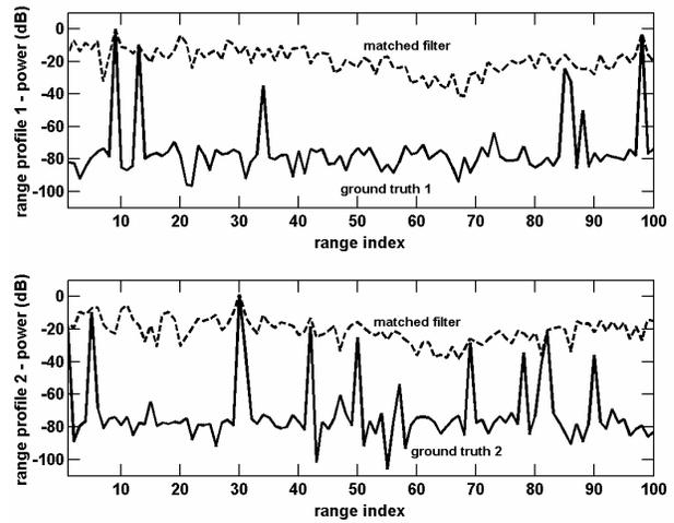
Fig. 6. Matched filter results for multistatic radar reception without spatial beamforming separation
