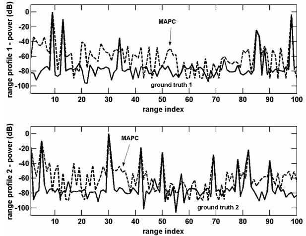
Fig. 7. MAPC results for multistatic radar reception without spatial beamforming separation
