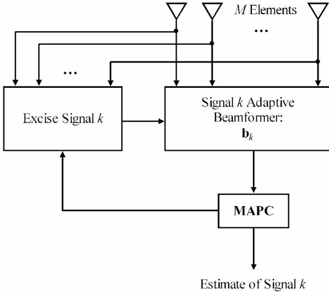
**Fig. 1.** MAPC-AB block diagram
