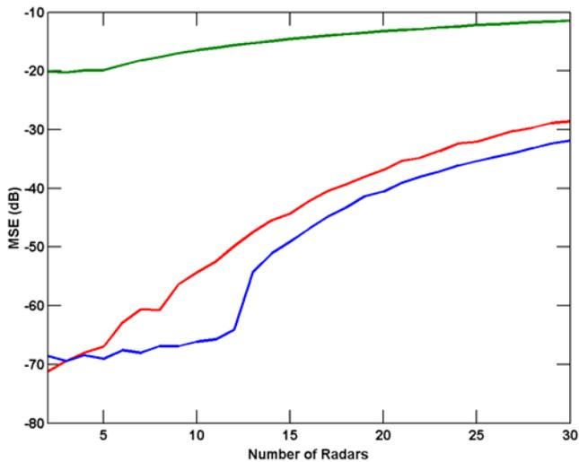
**Fig. 4.** Monte Carlo simulation for varying numbers of multistatic radars (green: matched filter, red: MAPC, blue: MAPC-AB).
