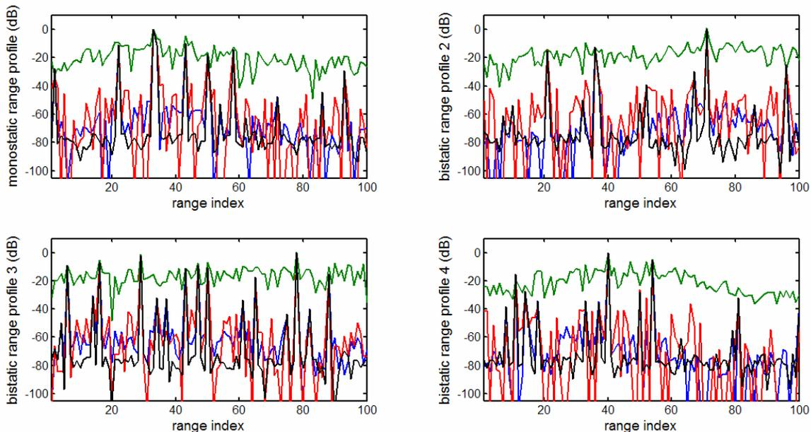
**Fig. 2.** Range profile estimation for multistatic radar reception (black: ground truth, green: matched filter, red: MAPC, blue: MAP-AB).
