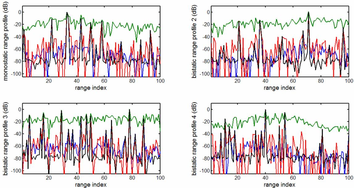
**Fig. 3.** Range profile estimation for multistatic radar reception with decreased angular separation between received signals (black: ground truth, green: matched filter, red: MAPC, blue: MAPC-AB).
