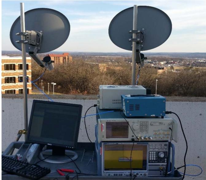
Figure 6. Hardware instrumentation setup for open-air measurements
