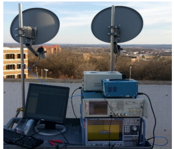
Fig. 3. Hardware instrumentation setup for open-air measurements
