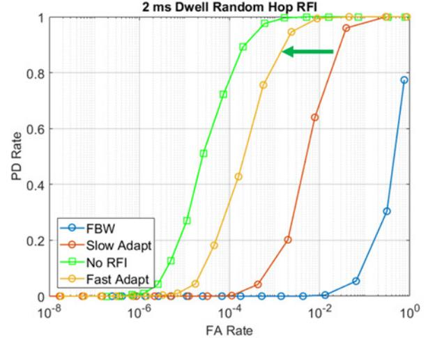
**Fig. 8: ROC curves where the SDRadar is adapting at 3.2 ms (“Slow Adapt”) and 160  $\mu$ s (“Fast Adapt”), while coexisting with randomly hopping RFI.**
