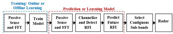
Fig. 2: General block diagram of the Sense-Predict-Avoid and Sense-Learn-Avoid approaches.
