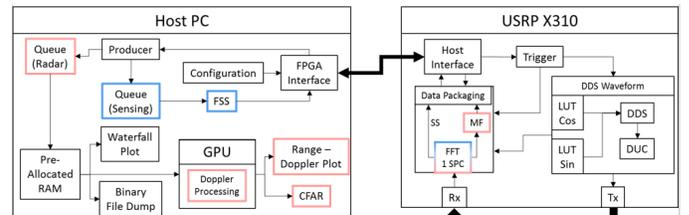
Fig. 6: Block diagram of the basic SDRadar for Sense-React-Avoid.
