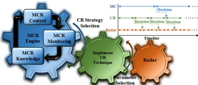
Fig. 9: Metacognitive radar model (MCR) to select the appropriate CR technique based on real-time observations of radar performance and the EME.
