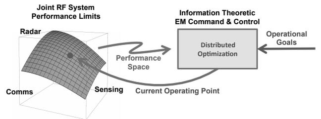
Fig. 3. Notional performance manifold for a joint radar, communications, and sensing system, and how this manifold influences system design and optimization decisions.
