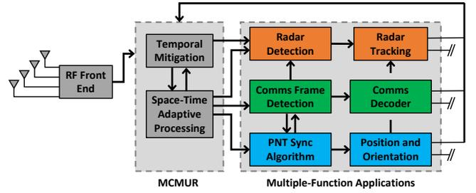
Fig. 7. Joint radar, communications, and PNT receiver processing chain. We extend the receiver architecture developed and validated in [4] to include radar processing and space-time adaptive processing techniques. This architecture would generally be considered impractical for real implementations, but we assert that the newest generation of domain-specific RF hardware platforms will begin to support this level of receiver processing.
