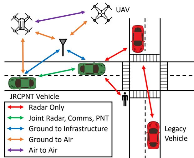
Fig. 1. Numerous vehicular applications benefit from simultaneous sensing and communications capabilities. PNT services offer extremely precise positioning and navigation capabilities, but radar systems are still critical for detecting and tracking uncooperative targets such as pedestrians or legacy vehicles. Integrated communications provides a feedback channel for the radar and PNT services, increasing performance and also improving security against cyberattack.
