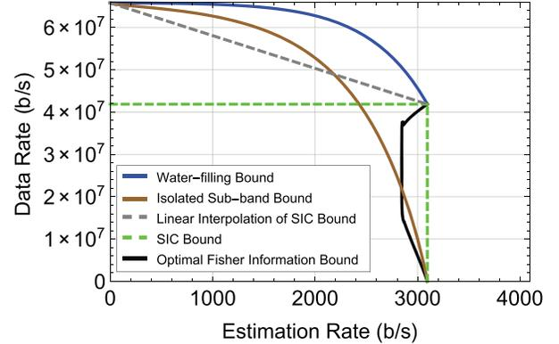
Fig. 2. Theoretical performance bounds for different radar-communications cooperation strategies, as derived in [2]. RF convergence techniques (successive interference cancellation, water-filling) simultaneously improve performance of both sub-systems.
