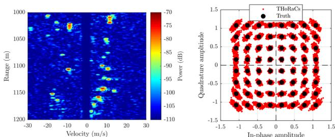
Fig. 4. Free-space experimental demonstration of THoRaCs dual-function radar/communication waveforms. (L) Range-Doppler response from moving vehicles traversing an intersection 1 km from the test setup. (R) Demodulated 64-QAM constellation at the intended receiver after synchronization and equalization [12].
