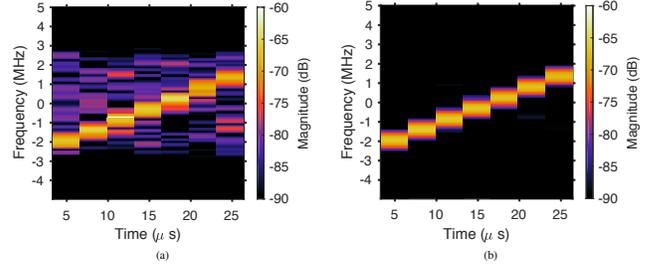
Fig. 8. Time frequency representation of in-band radar and communications users before and after successive interference cancellation. The communications signal is almost completely removed, allowing the radar system to process the return with essentially no interference.
