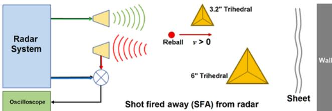
Fig. 4. Diagram of test setup showing the static targets and moving target within the radar's field of view.
