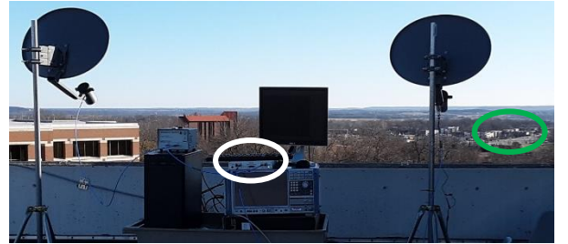
Fig. 4. Open-air test setup: Ettus x310 SDRadar (white oval) and illuminated traffic intersection (green oval)
