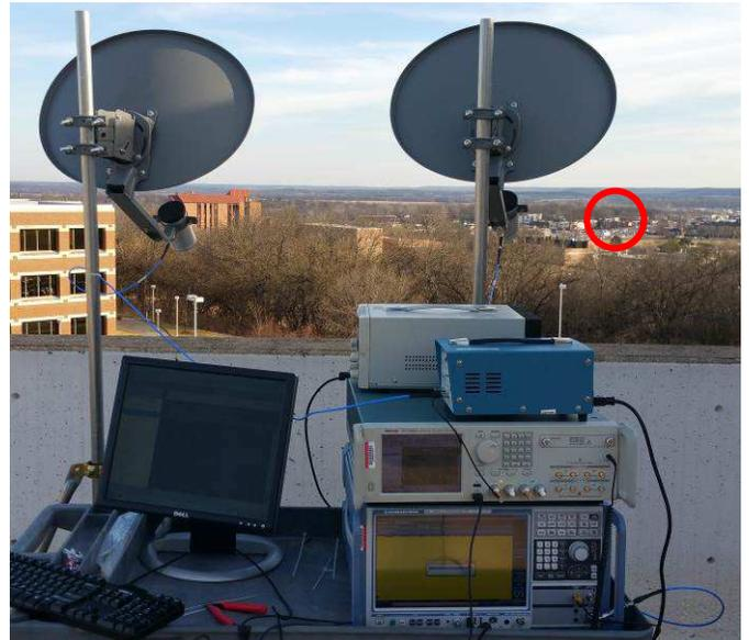
Fig. 6. Testbed for rooftop measurement of moving targets
