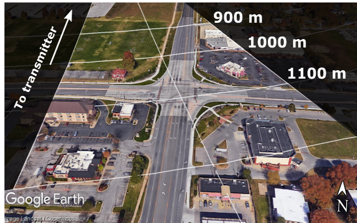
Figure 3.14: Field of view for open-air measurements with 12.3^\circ antenna beam
