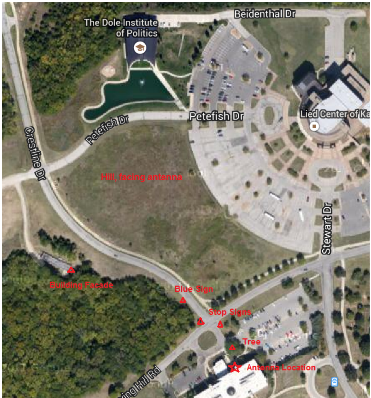
Figure 4.2: Radar field of view. The star near the bottom of the map gives the location of the antennas, and the targets that may produce significant reflections are denoted by triangles. The antennas are aimed at the Dole Institute of Politics, but given the beamwidth of the antennas, returns from the Lied Center are expected.
