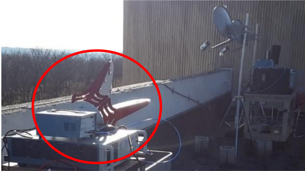
Figure 100: Open-air test setup: interference source (red oval)
