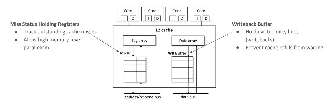
Cache internal structures are potential interference channels
