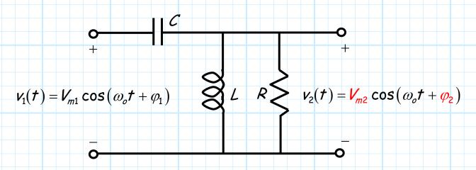
How do we determine the unknown magnitude  $V_{m2}$  and phase  $\varphi_2$  of this output?
