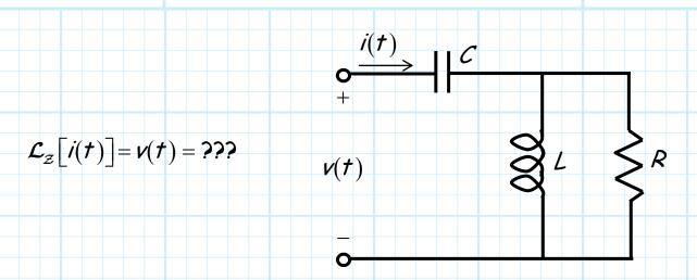
A: It turns out that any circuit constructed entirely with linear circuit elements is likewise a linear system (i.e., a linear circuit).
