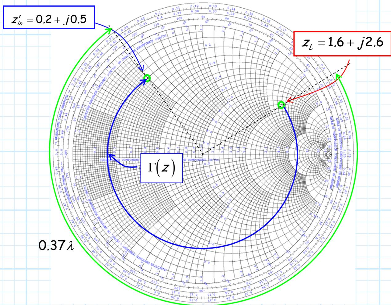
The **input impedance** is determined after rotating clockwise  $2\beta l$ , and is  $z'_{in} = 0.2 + j0.5$ .
