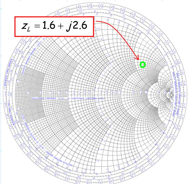
Then, we can rotate the **entire** Smith Chart  $180^\circ$  --while keeping the point  $\Gamma_L$  location on the complex  $\Gamma$  plane **fixed**.
