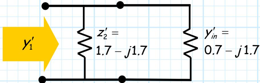
Determining  $y'_1$  is just **basic circuit theory**. We first express  $z'_2$  in terms of its admittance  $y'_2 = 1/z'_2$ .
