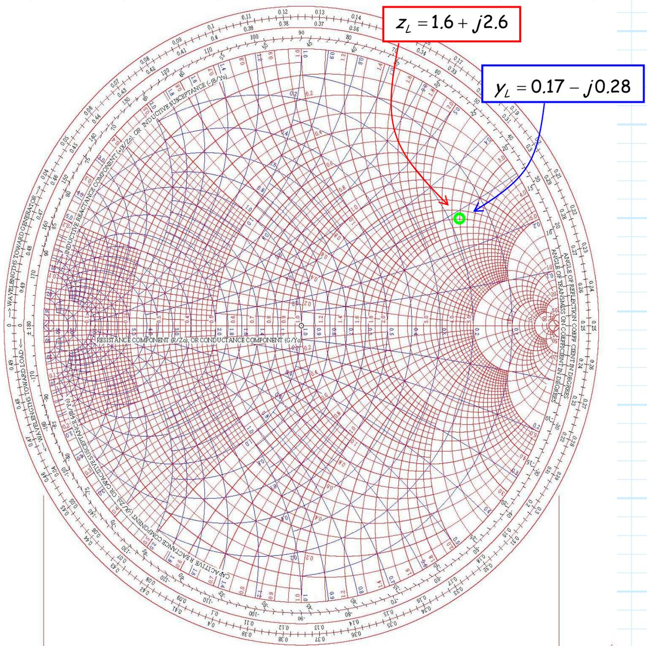
The Smith Chart above shows **both** the **impedance** mapping (red) and **admittance** mapping (blue). Thus, we can locate the impedance  $z_L = 1.6 + j2.6$  on the impedance (red) mapping, and then determine the value of that **same**  $\Gamma_L$  point using the admittance (blue) mapping.
