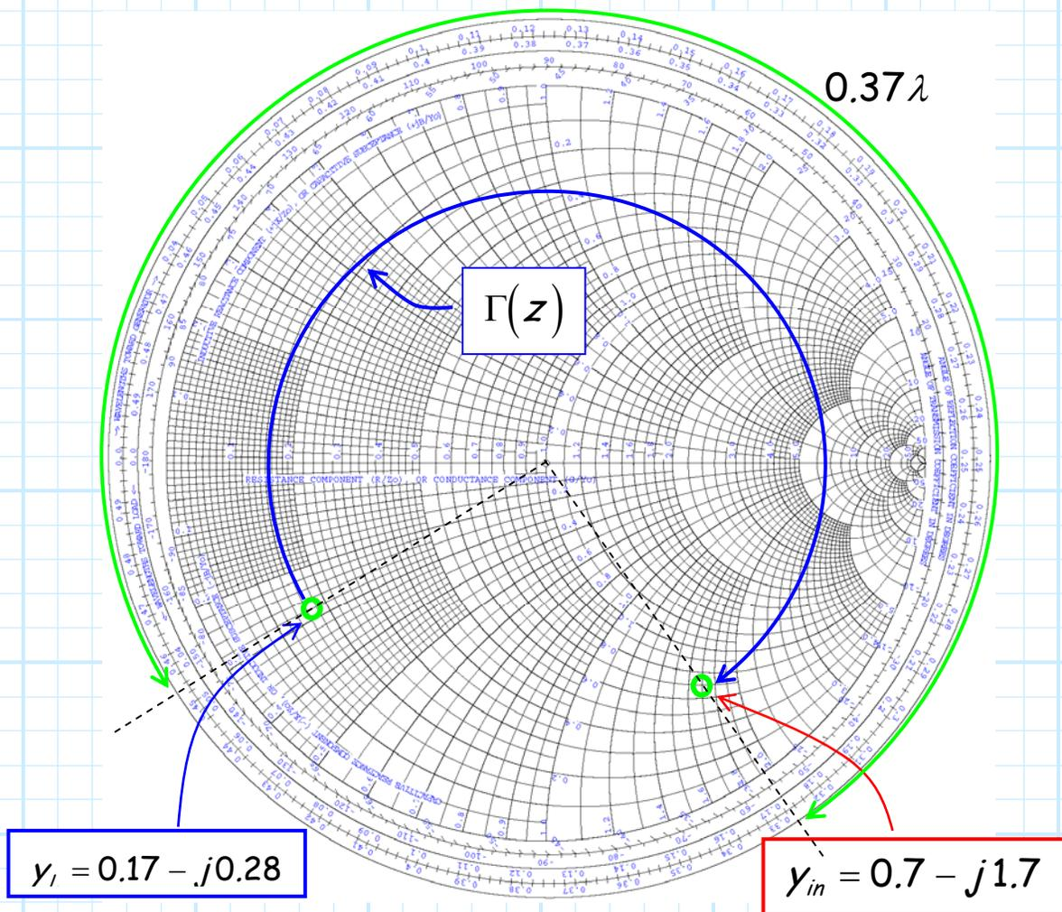
**Transforming** the load admittance to the beginning of the transmission line, we have determined that  $y'_{in} = 0.7 - j1.7$ .
