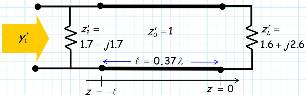
First, we need to determine the normalized **input** admittance of the transmission line:
