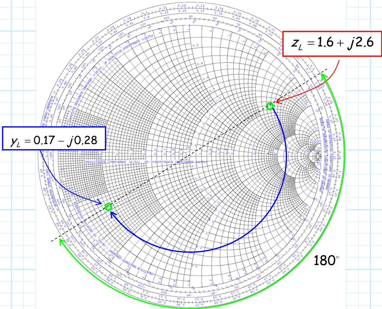
Now, we can determine the value of  $y'_{in}$  by simply **rotating** clockwise  $2\beta l$  from  $y'_L$ , where  $l = 0.37\lambda$ :
