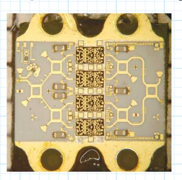
miniaturization technology. Microstrip circuits are constructed on ceramic or crystalline substrates, typically with low loss and high dielectric constant. Components such as chip resistors and conductors can be attached, as well as individual integrated circuits.
