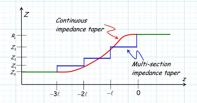
A tapered impedance matching network is defined by **two** characteristics—its **length** L and its taper **function**  $Z_1(z)$ :
