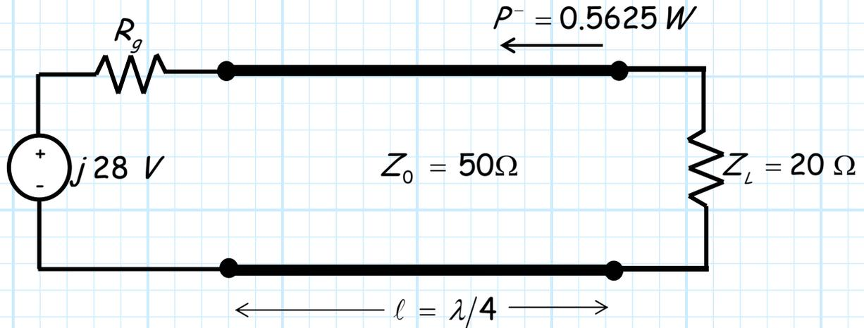
The **generator impedance** is purely real (i.e.,  $Z_g = R_g + j0$ )
