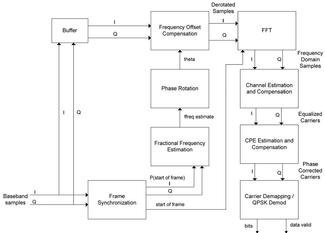
**Figure 3.2:** OFDM Receiver Block Diagram
