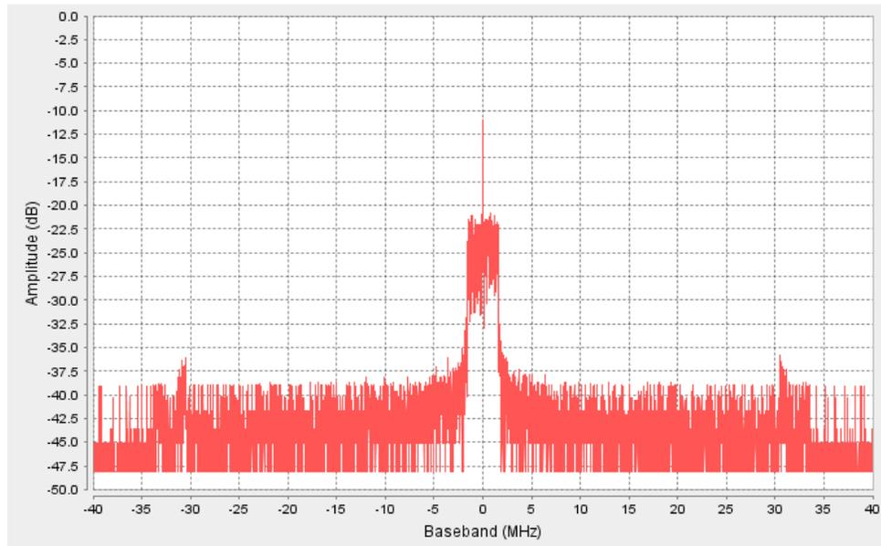
**Figure 4.27:** Received OFDM signal with 8x interpolating filter
