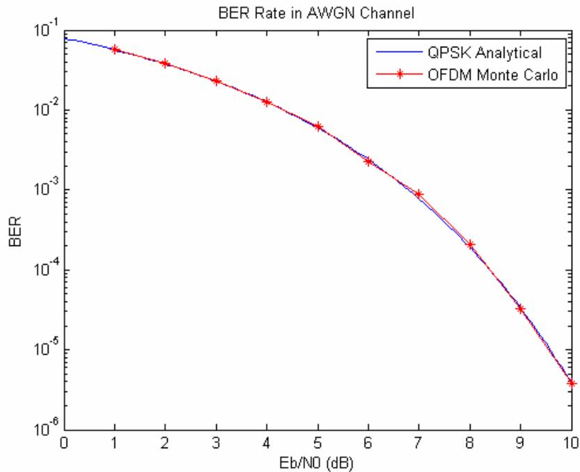
**Figure 4.23:** Validation for BER of OFDM design in pure AWGN channel
