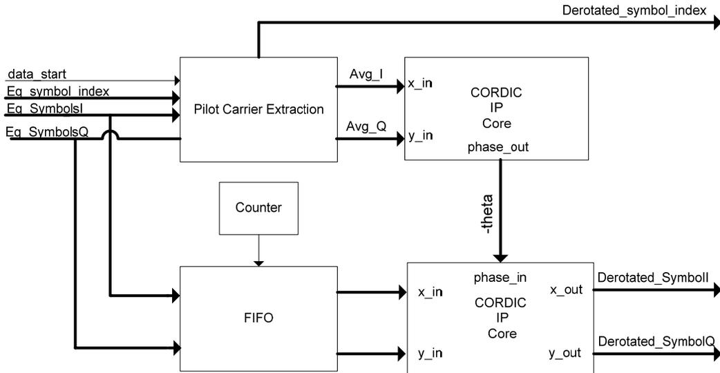
**Figure 4.17:** VHDL implementation of CPE estimation and compensation module
