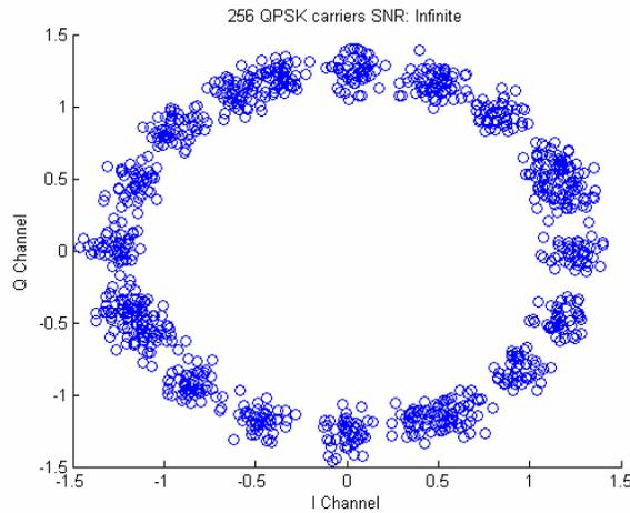
**Figure 2.9:** Uncompensated 0.05 subcarrier spacing frequency offset over 5 consecutive data symbols
