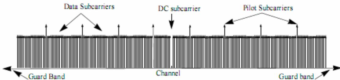
**Figure 3.3:** Illustration of the subcarrier assignments [2]
