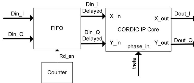
**Figure 4.11:** Implementation of Fractional Frequency Compensation Module
