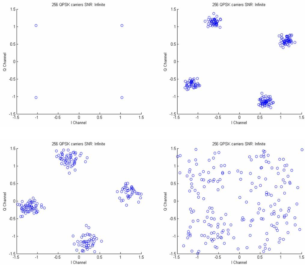
**Figure 2.8:** OFDM symbol with zero, 0.05, 0.1 and 0.25 subcarrier spacing fractional frequency offsets
