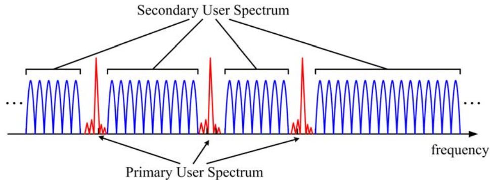
**Figure 2.1:** Illustration of an NC-OFDM system taking advantage of unused spectrum [14]
