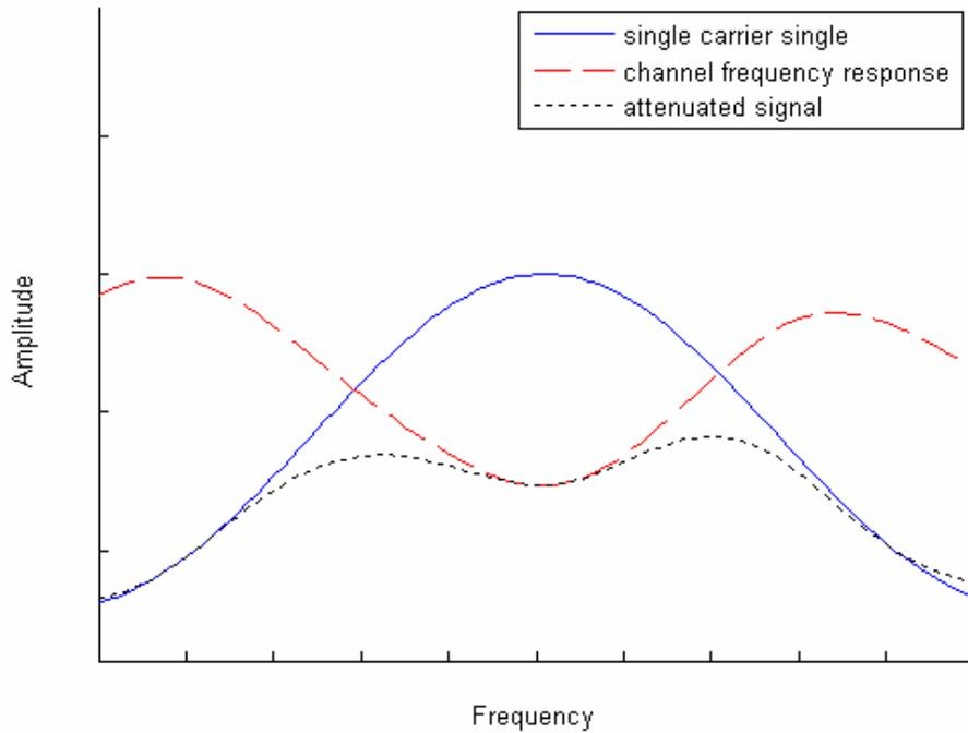
**Figure 2.4:** Single carrier signal undergoing frequency selective fading
