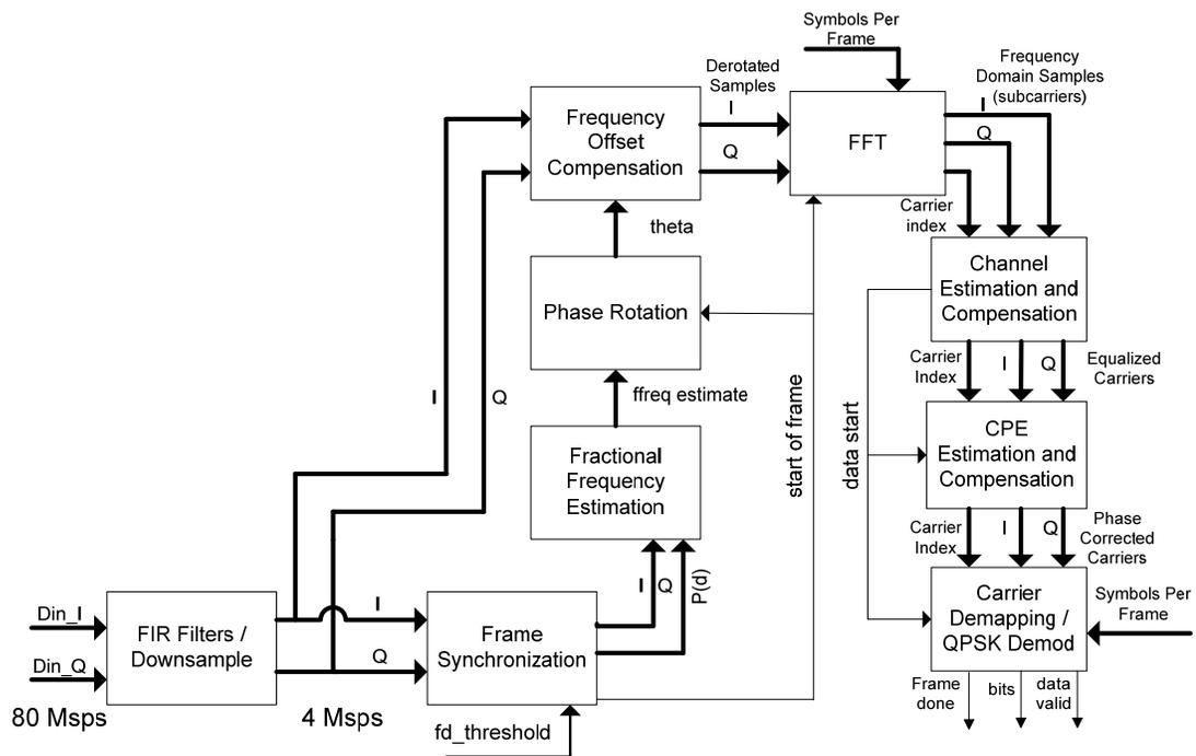
**Figure 4.3:** Receiver module top level design
