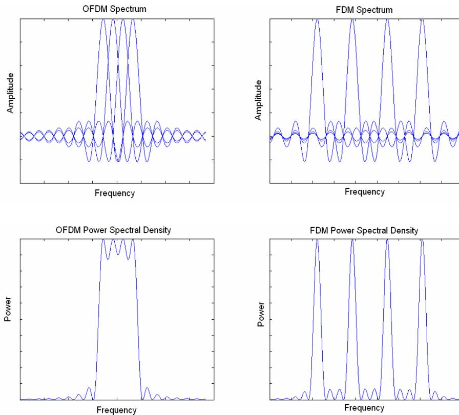
**Figure 2.3:** Spectrum and power spectral density of OFDM and FDM transmissions
