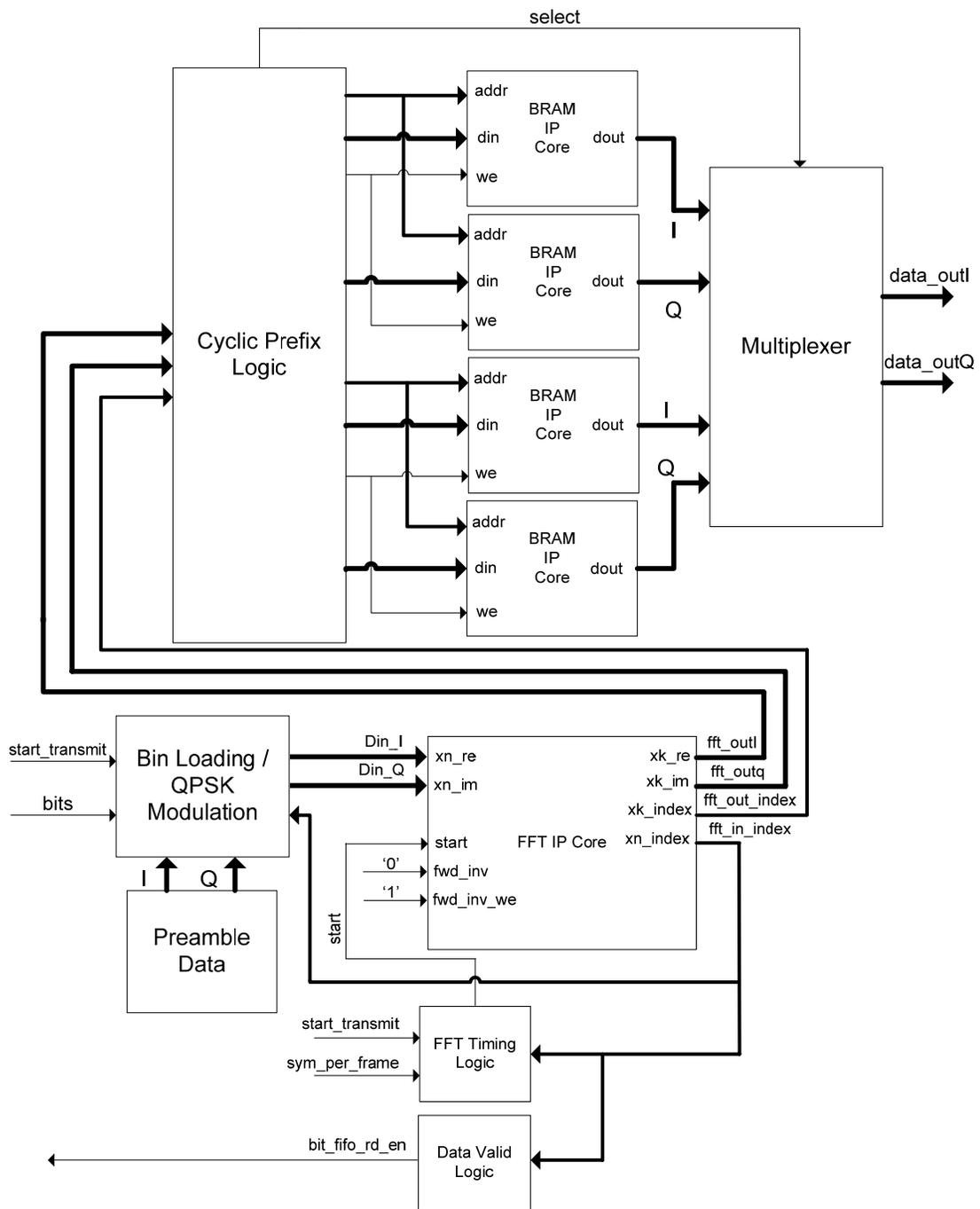
**Figure 4.22:** Detailed design of OFDM transmitter
