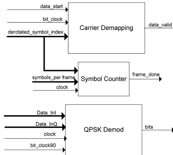
**Figure 4.19:** VHDL implementation of Carrier Demapping / QPSK demodulation module
