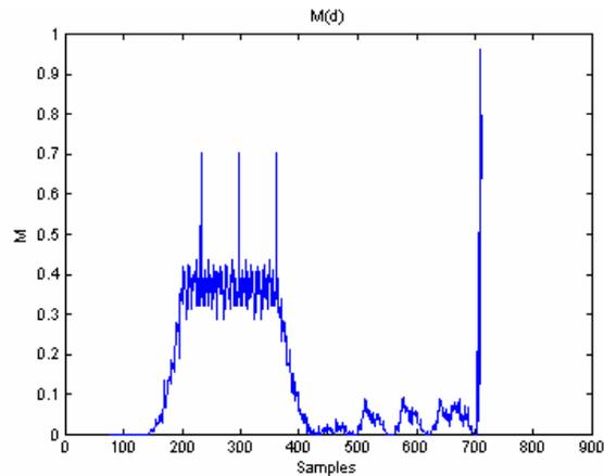
**Figure 3.6:** Kishore and Reddy algorithm operating in the absence of noise
