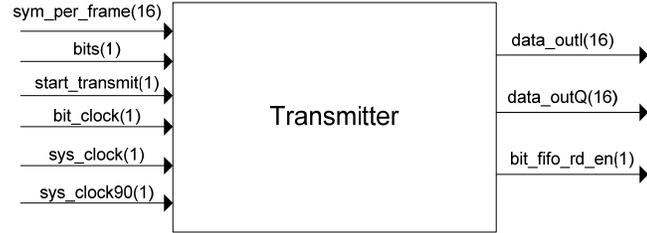
**Figure 4.20:** Port Map of VHDL Transmitter
