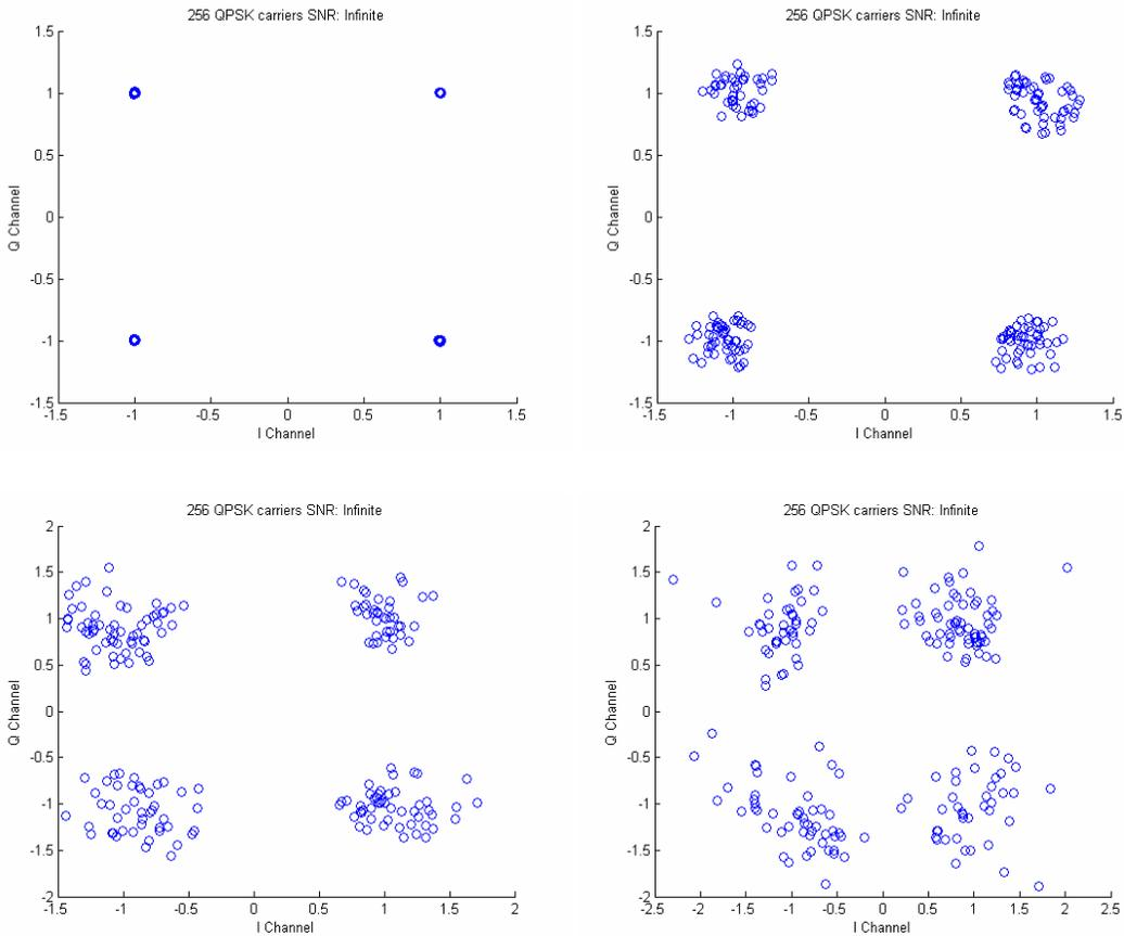
**Figure 3.13:** ISI due to integer timing offsets with proposed channel estimation algorithm for offsets of 0, 2, 5, and 10 samples respectively
