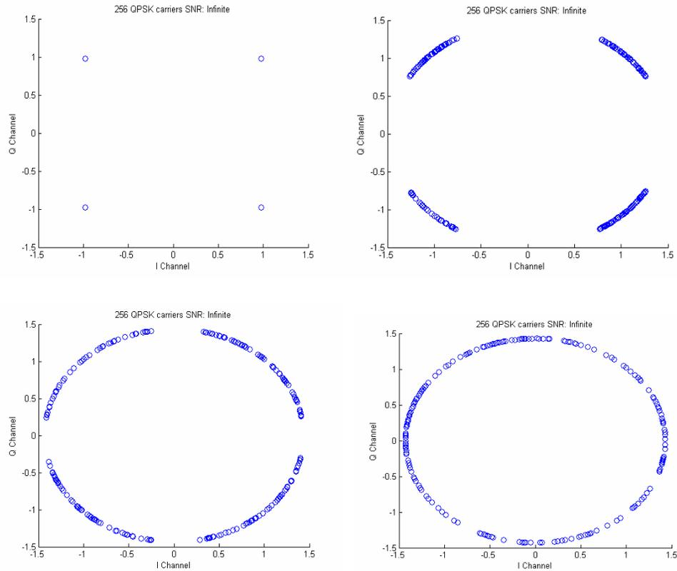
**Figure 2.6:** OFDM symbol with zero, 0.1, 0.25 and 0.5 sample period fractional timing offsets
