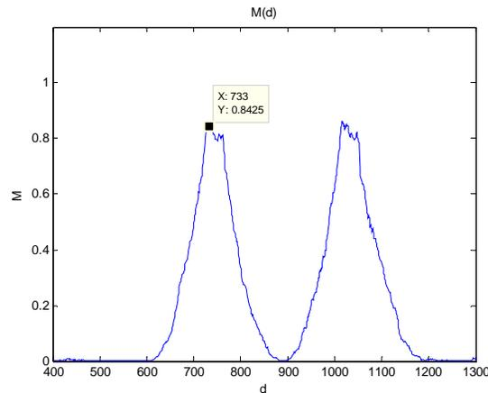
**Figure 3.9:** Schmidl and Cox algorithm operating at SNR = 10 dB
