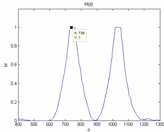
**Figure 3.8:** Schmidl and Cox algorithm operating in the absence of noise
