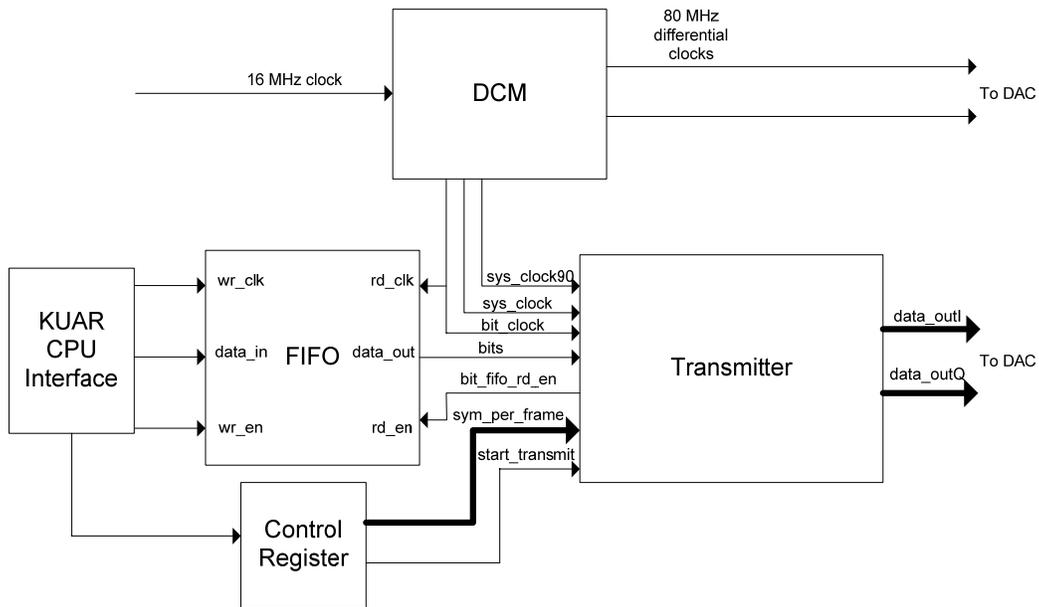
**Figure 4.21:** Top level FPGA design for OFDM transmitter
