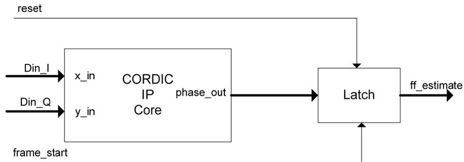
**Figure 4.7:** Implementation of Fractional Frequency Estimation Module
