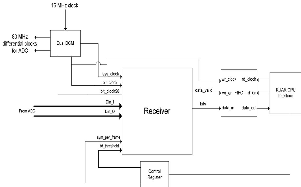
**Figure 4.2:** External logic for top-level FPGA design
