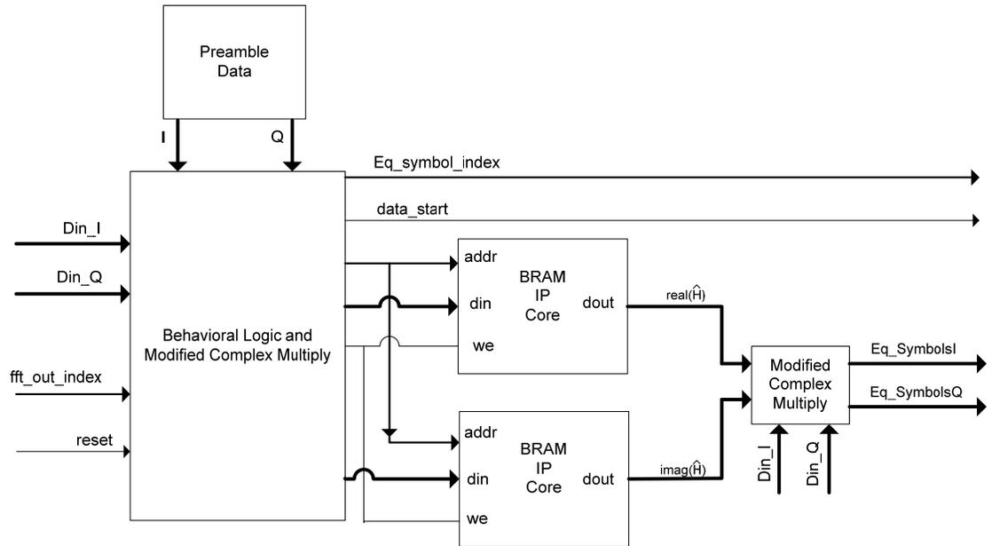
**Figure 4.15:** Implementation of Channel Estimation and Equalization module
