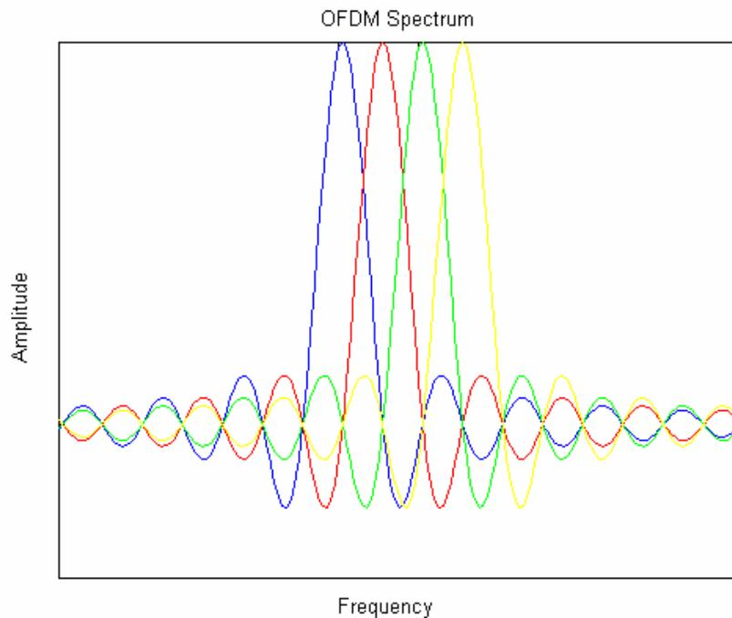
**Figure 1.2:** Four subcarrier OFDM spectrum
