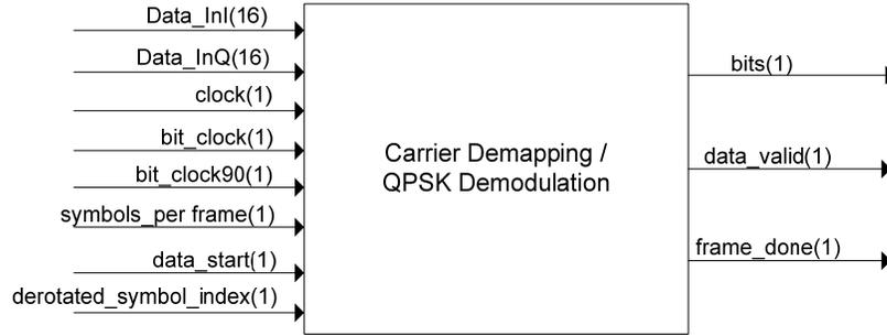
**Figure 4.18:** Carrier Demapping / QPSK Demodulation module port map
