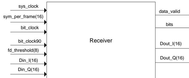
**Figure 4.1:** Receiver module port map
