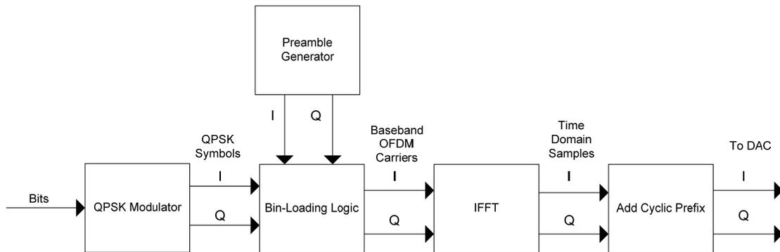
**Figure 3.1:** OFDM Transmitter Block Diagram
