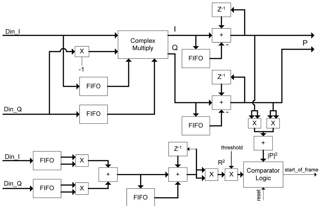
**Figure 4.5:** Implementation of Frame Synchronization Module
