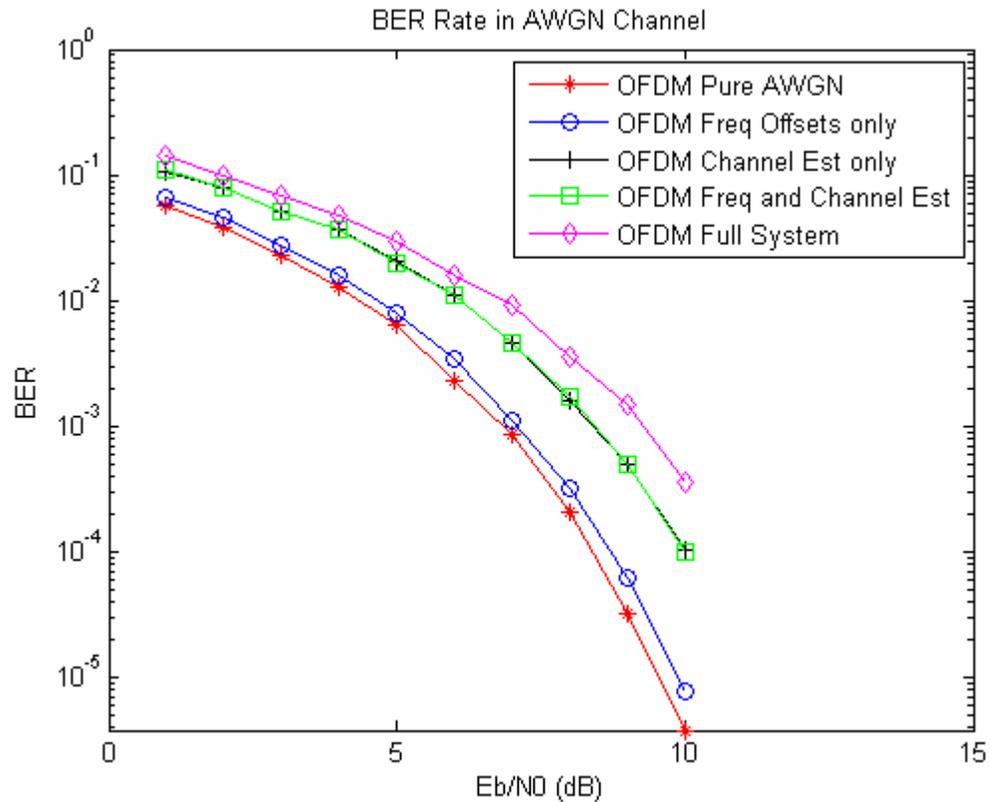
**Figure 4.24:** BER performance of Matlab simulations
