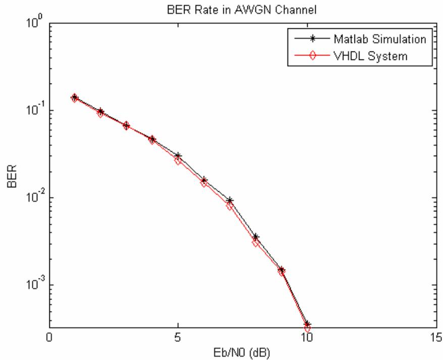
**Figure 4.25:** VHDL system versus Matlab simulation BER
