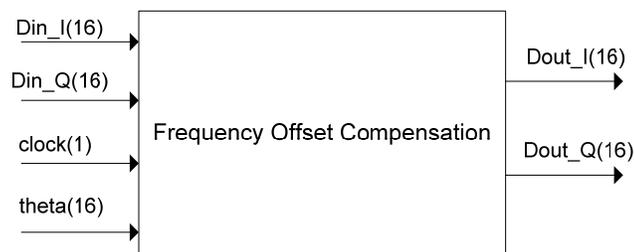
**Figure 4.10:** Frequency offset compensation module inputs and outputs
