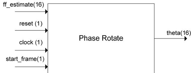
**Figure 4.8:** Phase rotation module input and output ports
