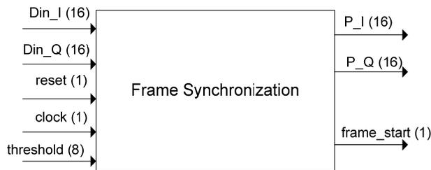
**Figure 4.4:** Inputs and outputs of the frame synchronization module
