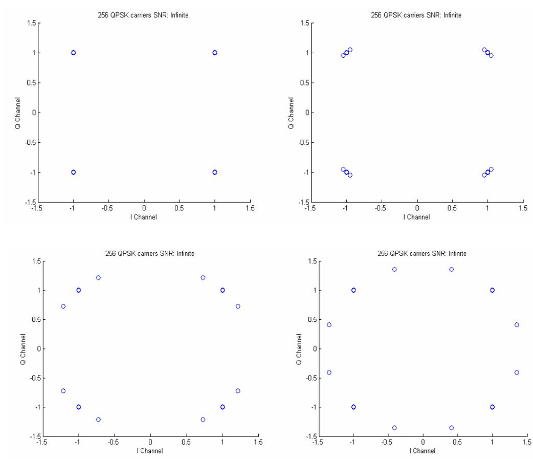
**Figure 3.12:** Residual carrier rotations to due integer timing frequency offsets with proposed channel estimation algorithm for offsets of 0, -2, -10, and -20 samples respectively.
