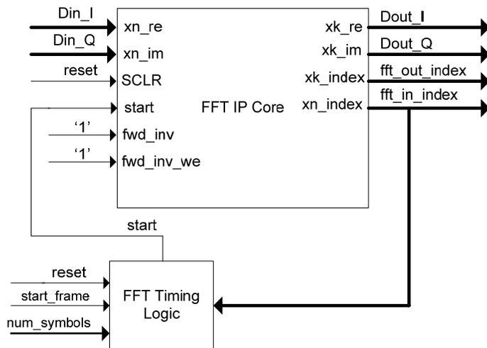
**Figure 4.13:** Implementation of FFT module
