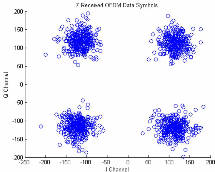
**Figure 4.28:** KUAR “across the room” laboratory transmission and reception of 1 frame including 7 OFDM data symbols. 2688 bits, BER = 0.
