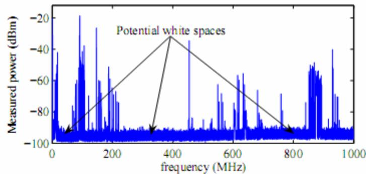
**Figure 1.1:** Spectrum measurement from 900 kHz to 1 GHz [5]
