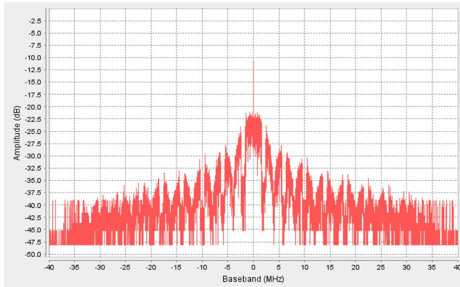
**Figure 4.26:** Received OFDM signal with no filtering
