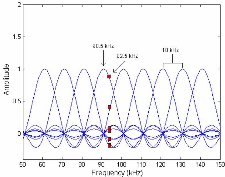
**Figure 2.7:** Inter-carrier interference caused by a frequency offset of 20% of a subcarrier spacing
