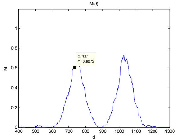
**Figure 3.10:** Schmidl and Cox algorithm operating at SNR = 5 dB
