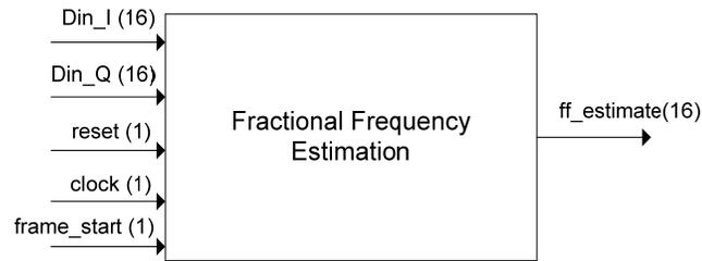
**Figure 4.6:** Inputs and outputs of the fractional frequency estimation module
