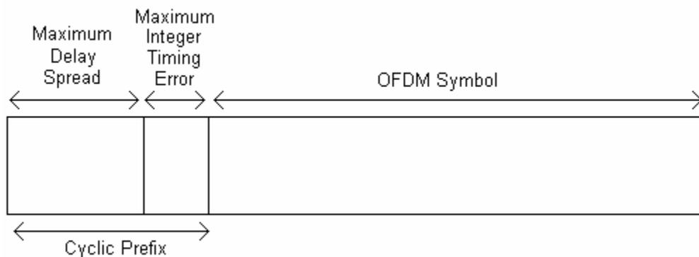
**Figure 3.11:** Accounting for the maximum integer timing error in the cyclic prefix
