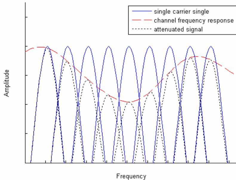
**Figure 2.5:** Approximately flat fading sub-channels in a frequency selective channel
