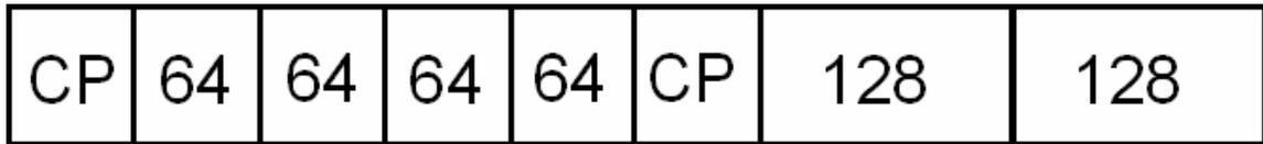
**Figure 3.5:** Time domain representation of full preamble
