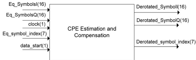
**Figure 4.16:** CPE estimation and compensation module port map
