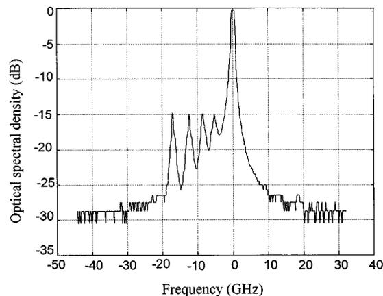
Fig. 3. Measured SSB optical spectrum with four subcarrier channels.
