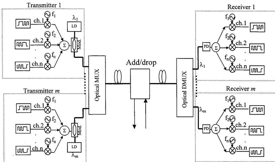
Fig. 1. SCM/WDM system architecture.
