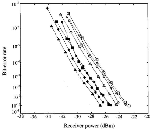
Fig. 4. Measured BER in a system with 4 subcarrier channels before (solid points) and after (open points) a fiber transmission line with a  $-2640$  ps/nm total dispersion.
