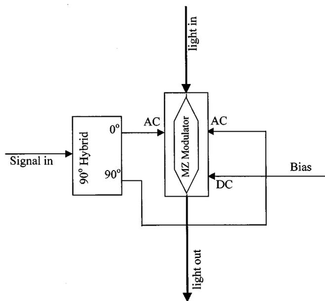
Fig. 2. Optical SSB modulation using dual-electrode MZM.
