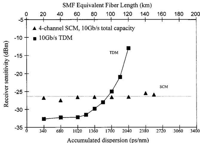
Fig. 5. Receiver sensitivity (at BER of  $10^{-9}$ ) comparison between a 10-Gb/s TDM system and a four-tone SCM system with 10-Gb/s capacity.
