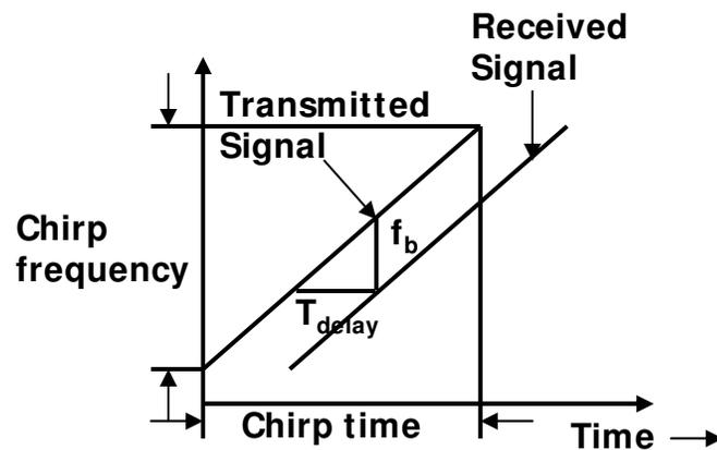
$$\frac{f_b}{BW} = \frac{T_{delay}}{t_{chirp}}$$
