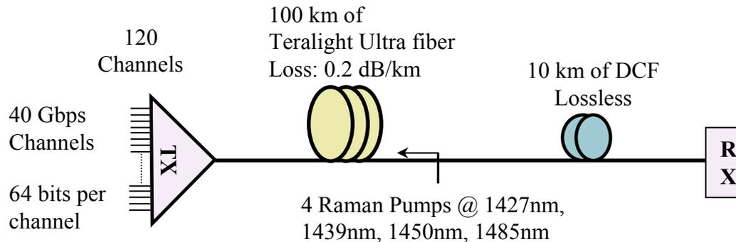
$$Gain(dB) = \text{AttenuationParameter} * \text{Length} + 10 * \log\left(\frac{P_{avg,out}}{P_{avg,in}}\right)$$
