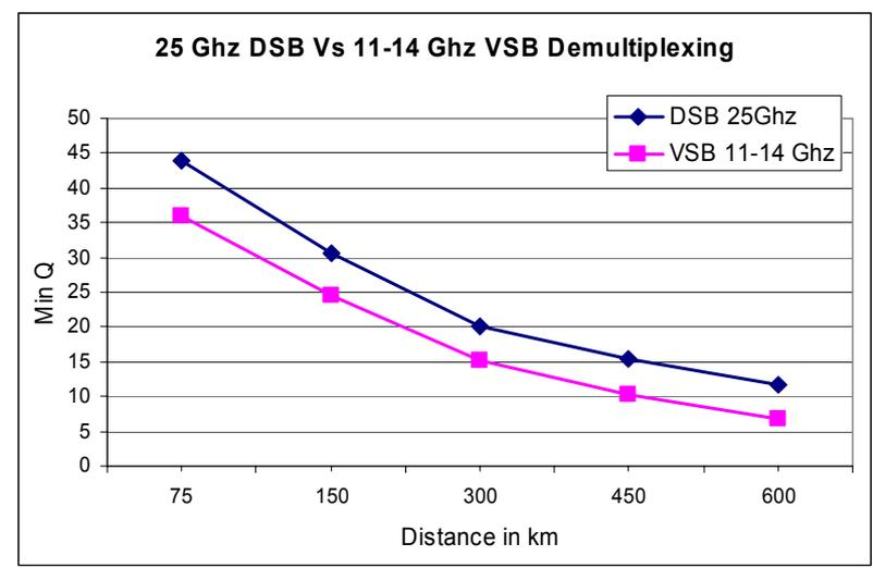
Channel launch power used is 1.5 mW
