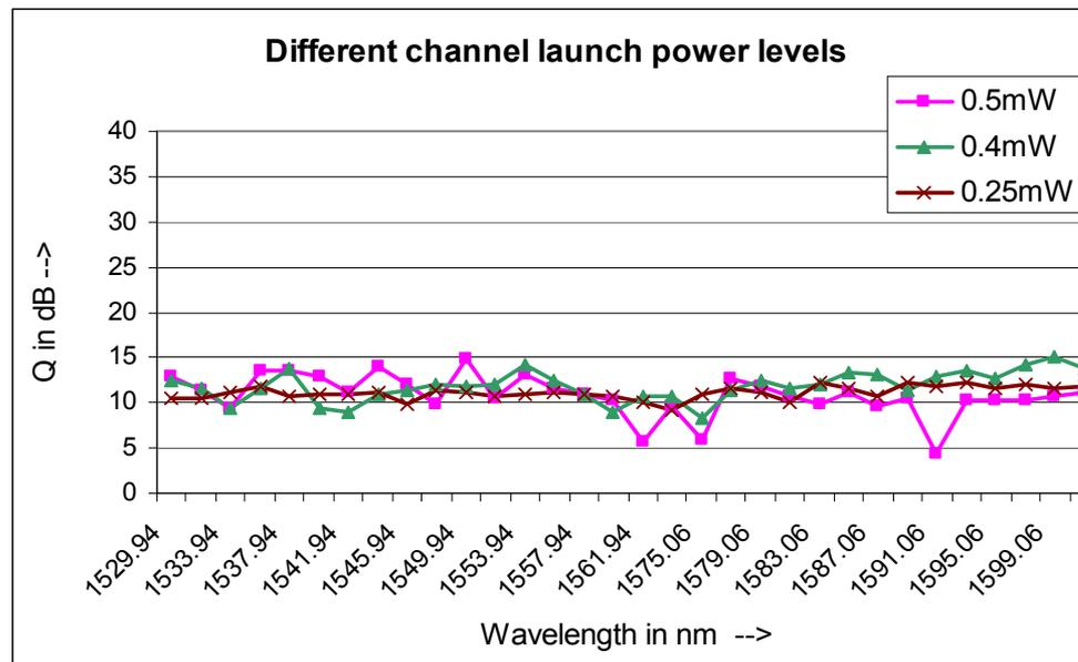
System performance at the end of 1200 km for different channel launch powers
