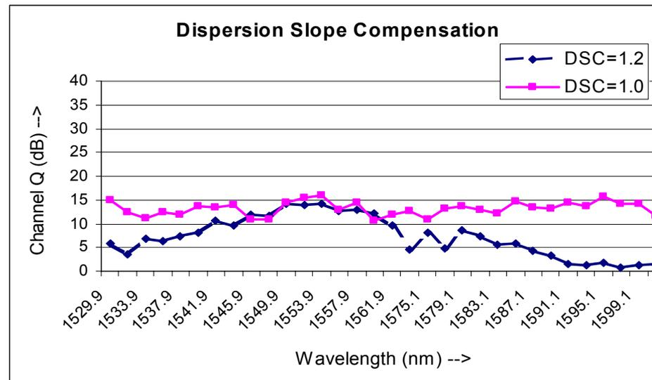
System performance at the end of 1200 km with and without dispersion slope compensation
