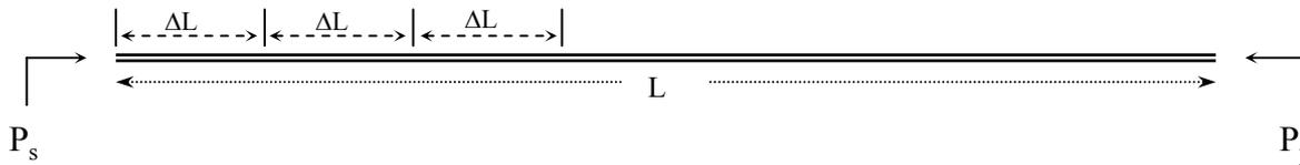
$$I_s(\Delta L) = I_s(0) \exp \{ g_R I_0(\Delta L) L_{eff} - \alpha \cdot \Delta L \}$$
