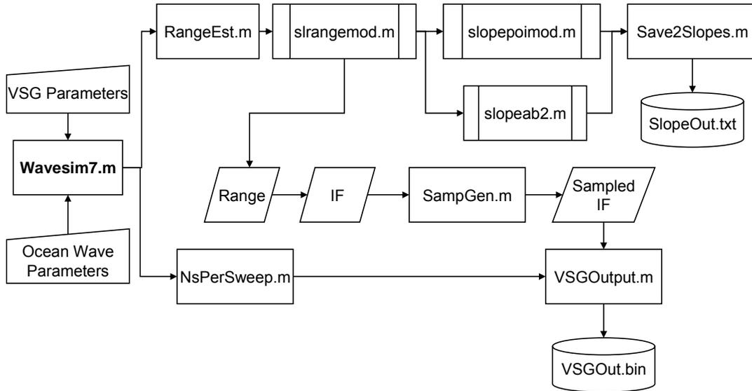
Figure 4.2. Wavesim7.m Block Diagram
