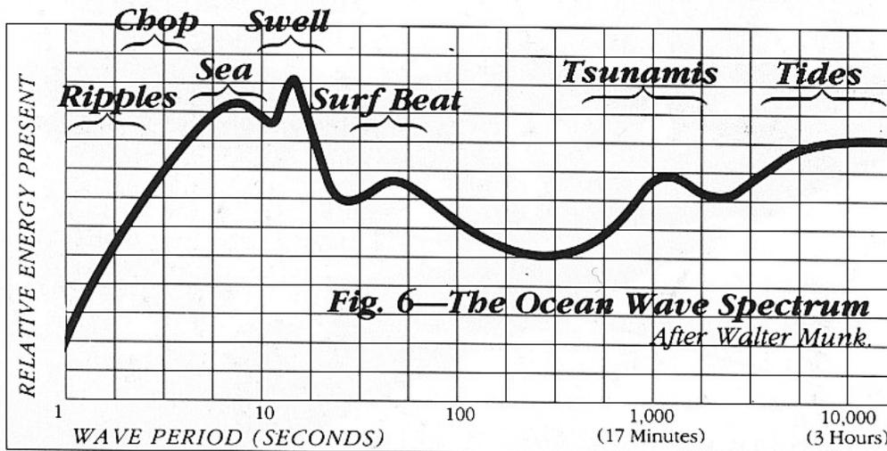
Figure 2.2. Ocean Wave Energy Spectrum
