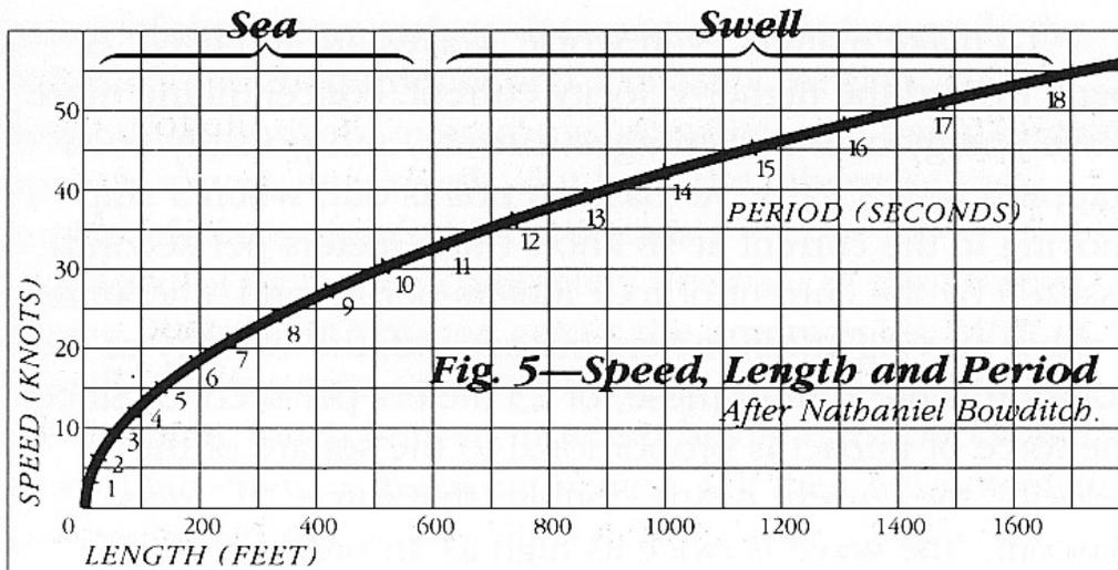
Figure 2.3. Wave Speed vs. Wave Length with Period.
