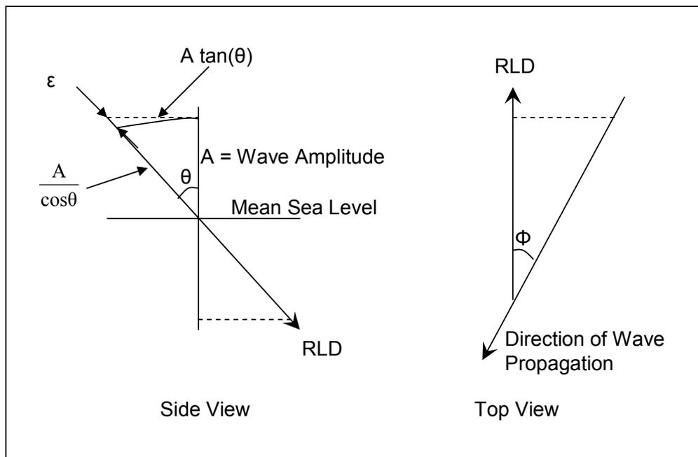
Figure 4.3. Geometry used to calculate phase and range error in a single beam due to slant range measurement. Adapted from (Evans, 1994).
