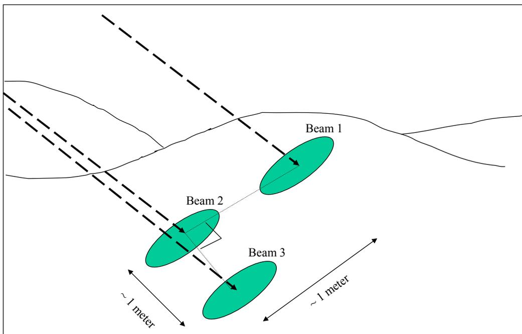
Figure 3.1. Beam Spot Arrangement on Ocean Surface
