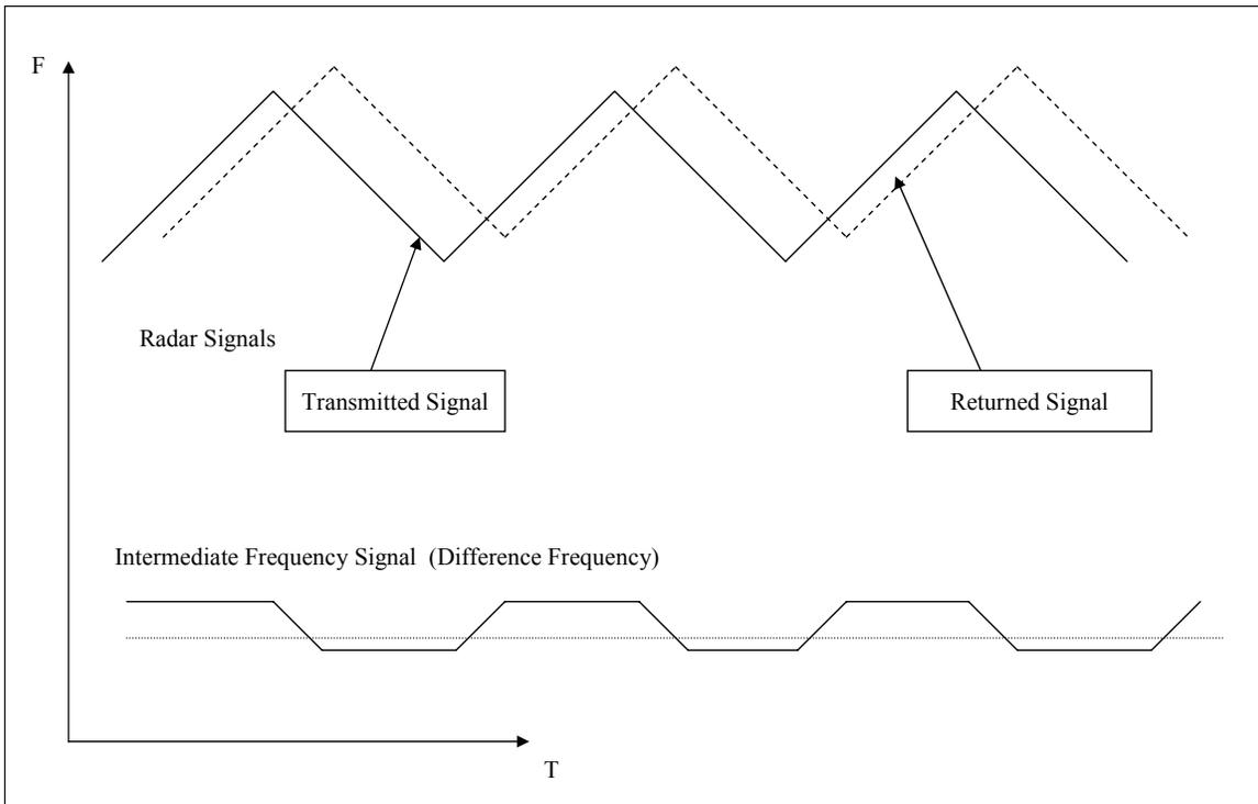
Figure 3.4. FM Radar Return from a Point Target with Doppler Shift Added
