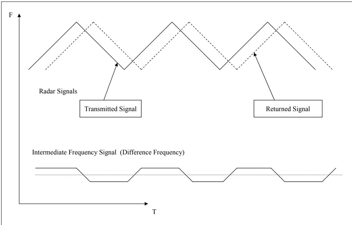
Figure 3.3. FM Radar Return from a Point Target
