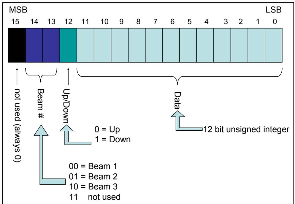
Figure 4.1. Digital VSG Data Output Structure
