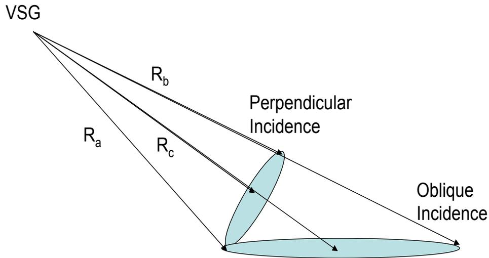
Figure 4.4. Illustration of Range/Frequency Spreading In an FM Radar
