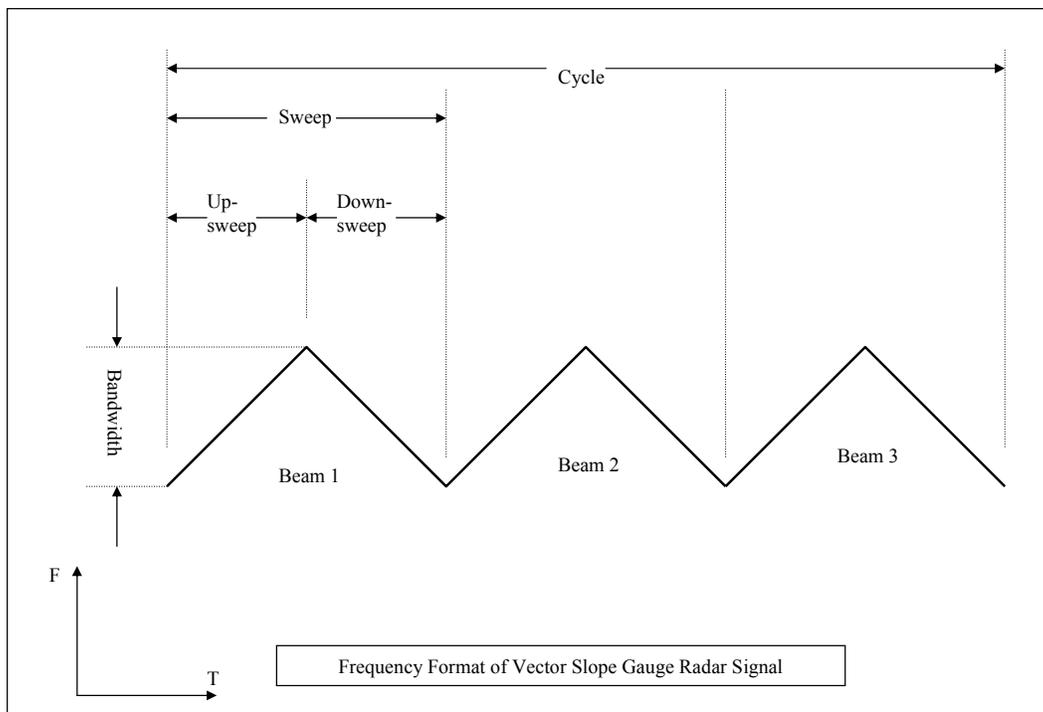
Figure 3.2. Frequency Format of VSG Radar Transmitted Signal
