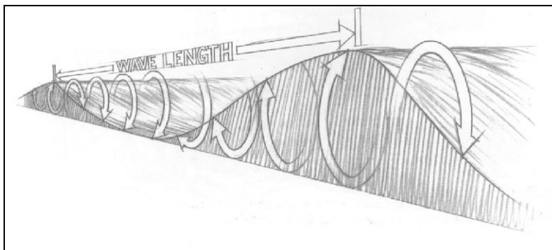
Figure 2.4. Orbital Motion in Approaching Wave [Kampion, 1997]
