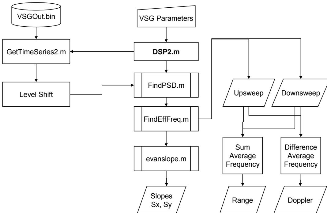
Figure 5.1. DSP2.m Block Diagram
