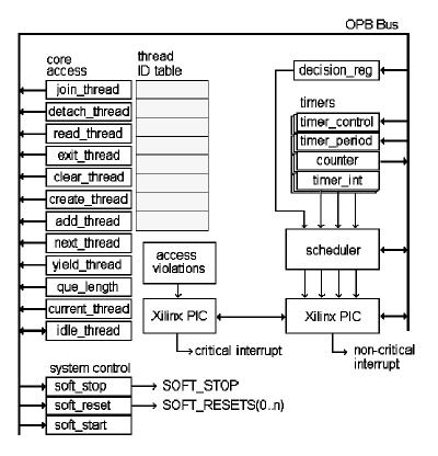
The diagram to the right shows the initial platform used to test the operation of the SWTM. The timers, decision\_reg, scheduler, and Xilinx PICs are not part of the SWTM but were added to create a minimal platform for evaluation and further development.
