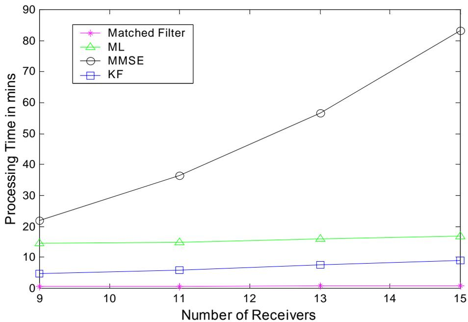
**Figure 3.10 Matched, ML, MMSE and Kalman Filters processing speed versus number of receive apertures for a sparse, random array**
