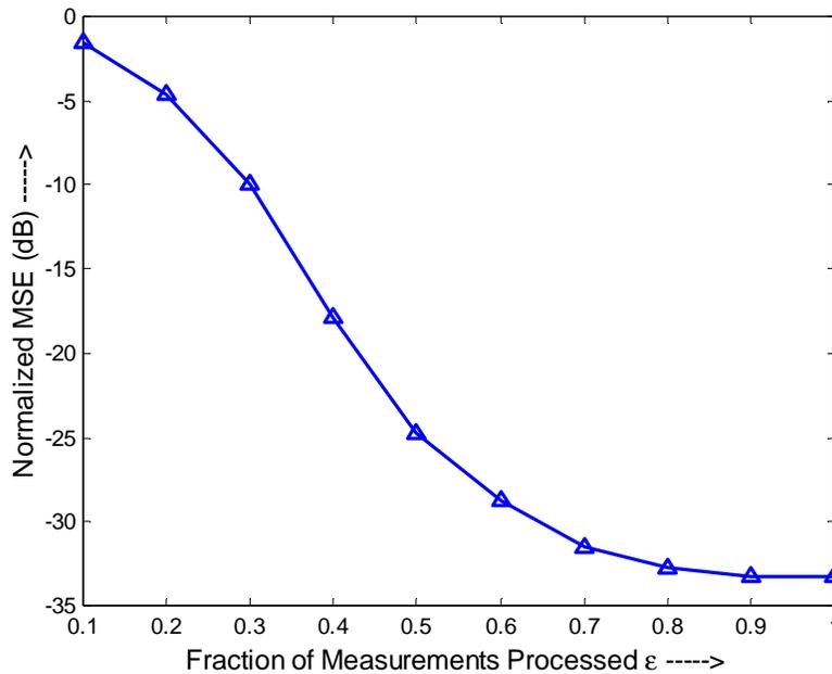
Figure 4.1 Normalized MSE (dB) vs. the fraction of Measurements Processed ( $\epsilon$ ) for the smaller version of the KU Football Stadium Image
