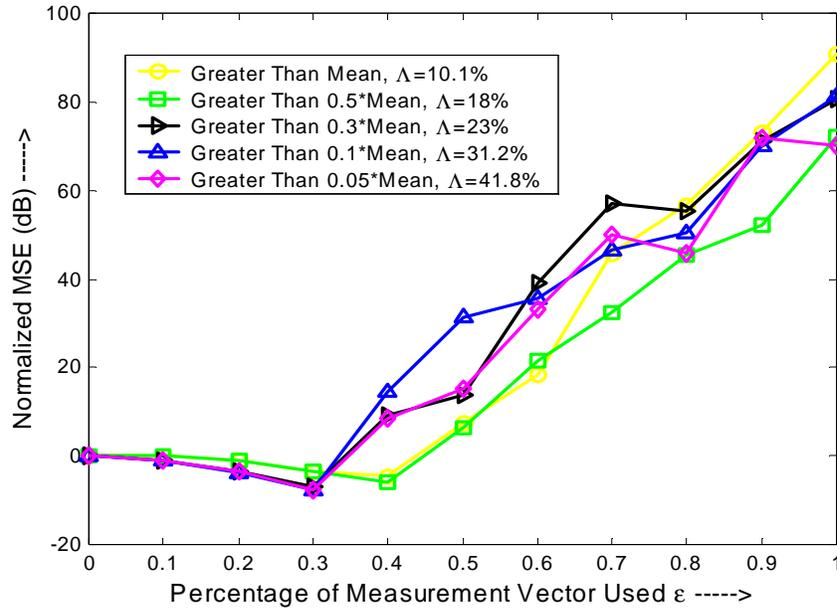
Figure 5.16 Normalized MSE versus the fraction of measurement data processed, for different thresholds
