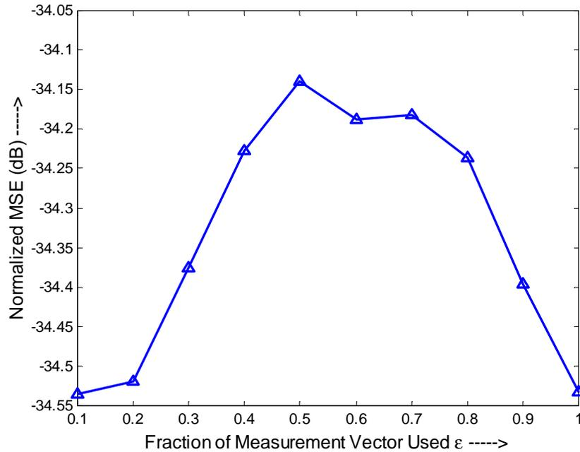
**Figure 4.9 Variation of Normalized MSE versus the fraction of measurement data processed for a case where the final values obtained for  $\mathbf{g}$  and  $\mathbf{K}_g$  are taken as the initial values and the processing is done again.**
