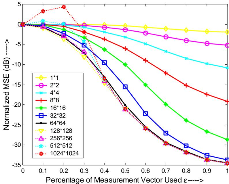
Figure 4.7 Variation of Normalized MSE versus the fraction of measurement data processed for processing, for different  $\mathbf{s}^2$  values for diagonal matrix  $\mathbf{K}_g(0)$
