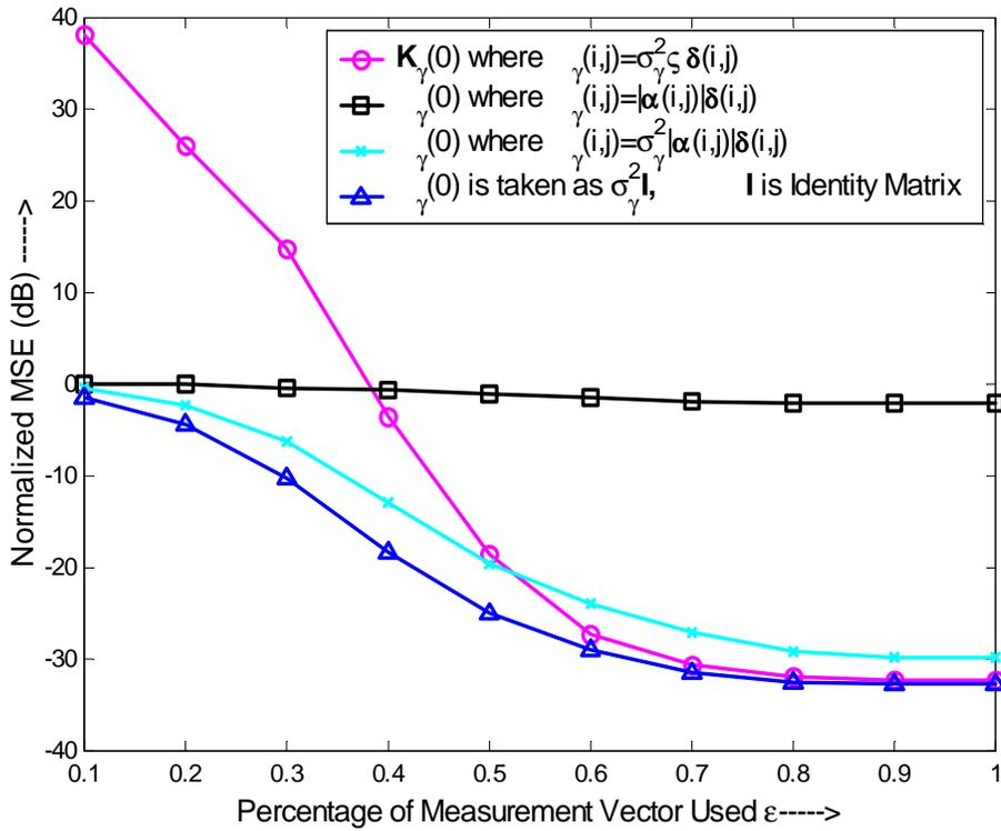
Figure 4.8 Variation of Normalized MSE versus the fraction of measurement data processed for processing for different  $K_g(0)$
