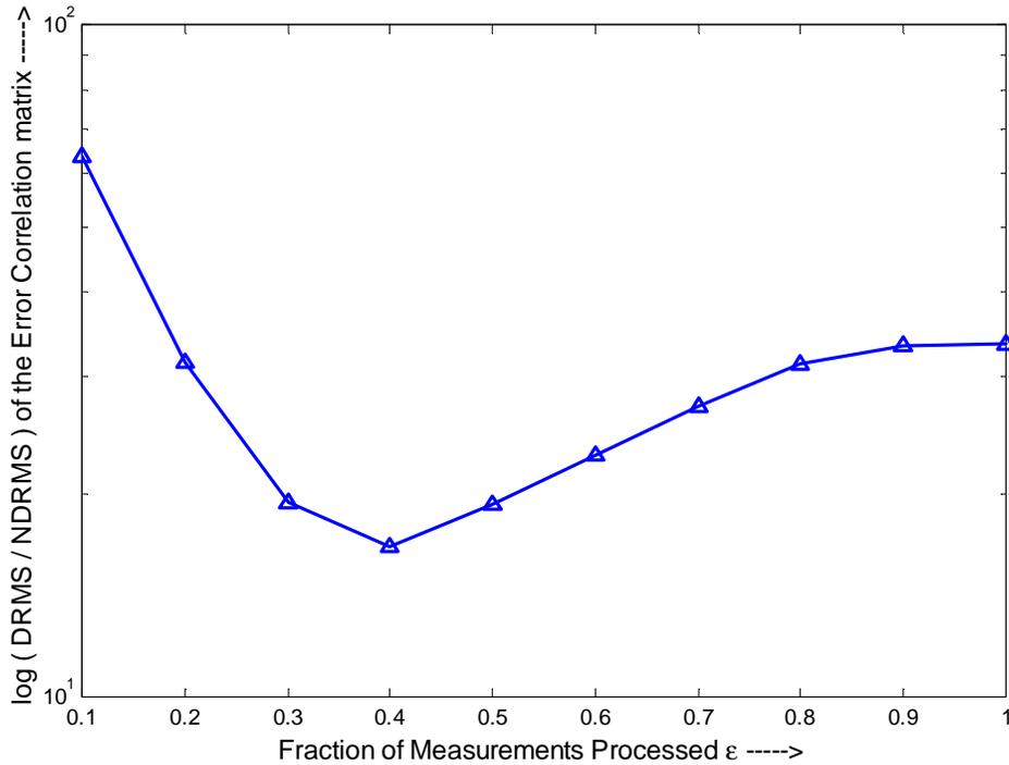
**Figure 4.3 Shows the Variation of the ratio between the RMS values of the diagonal and non-diagonal elements of the error correlation matrix**
