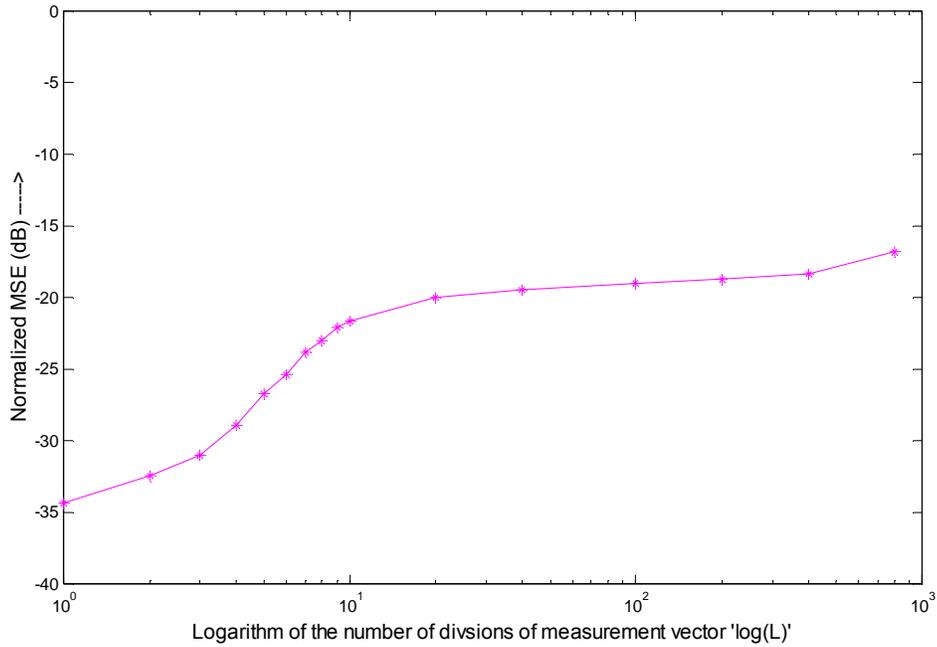
**Figure 5.10 Normalized MSE (dB) versus L for a case where only the diagonal elements are updated in the  $K_g$  matrix**
