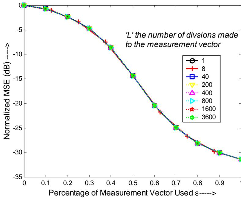
**Figure 4.6 Normalized MSE versus the fraction of measurement data processed for different L**
