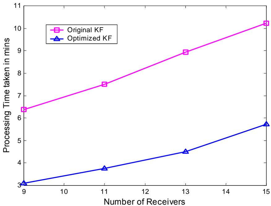
**Figure 5.4 Comparison between performance of optimized and unoptimized KF versus number of receive apertures in the sparse satellite cluster**
