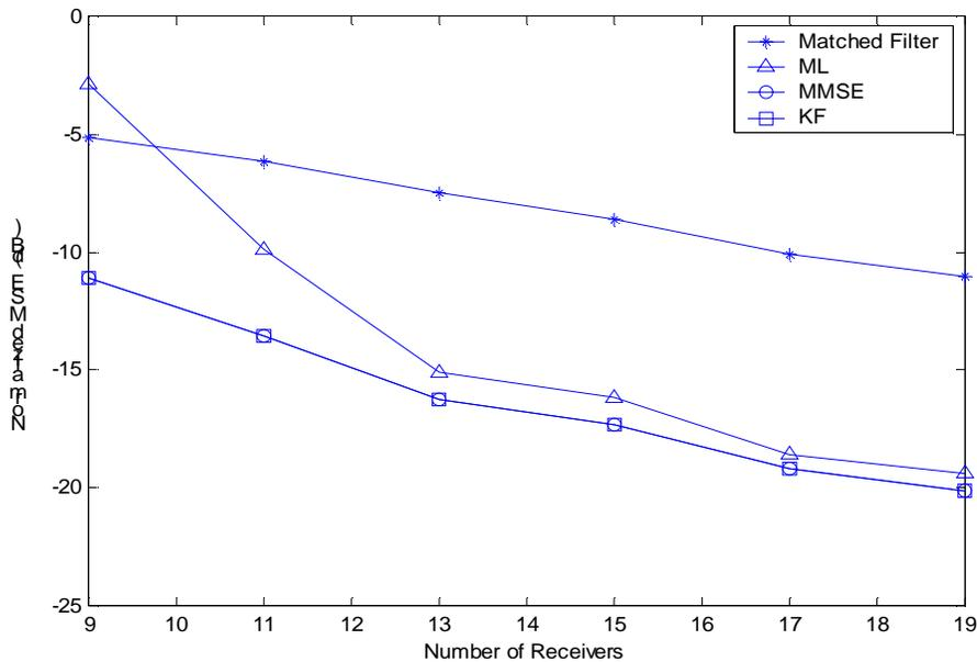
**Figure 3.9 Matched, ML, MMSE and Kalman Filters performance versus number of receive apertures for a sparse, random array and moderate SNR**
