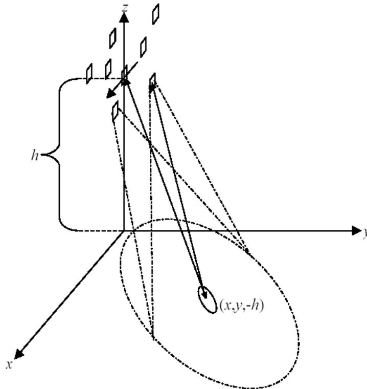
Figure 2.1 Radar Geometry for a constellation of radar satellites with the flat earth approximation [8]
