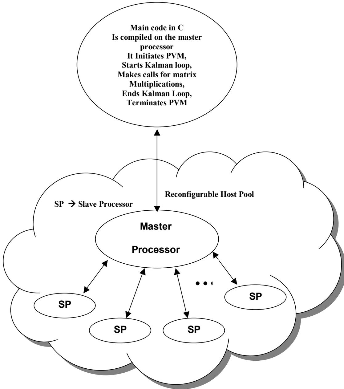
Figure 6.1 Diagram depicting the Parallel processing structure implemented in KF
