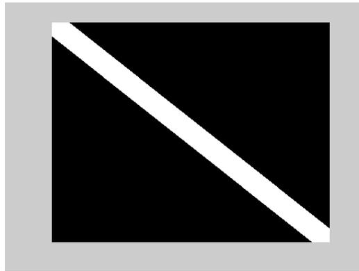
**Figure 5.13 Elements of  $\mathbf{K}_g$  considered for a diagonal spread consisting of 129 lines adjacent to the diagonal on either side**
