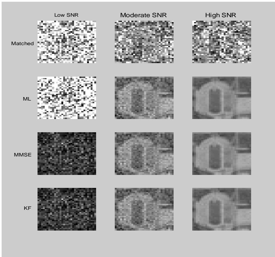
**Figure 3.7 Comparison of Matched, ML, MMSE and Kalman filters performance versus SNR**
