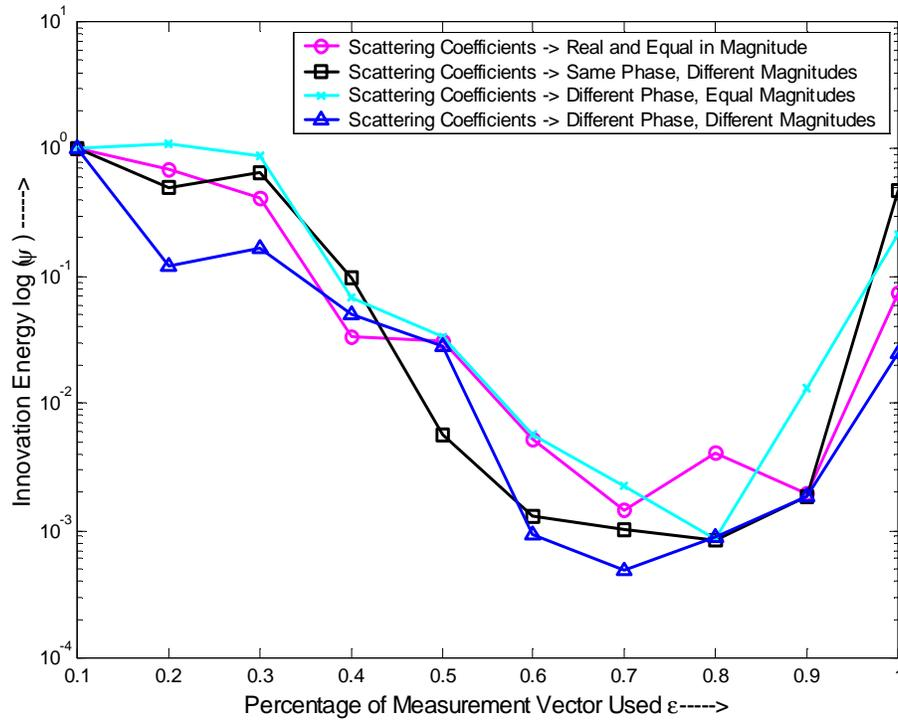
Figure 5.6 Innovation Energy vs. the fraction of measurement data processed for random scattering coefficients
