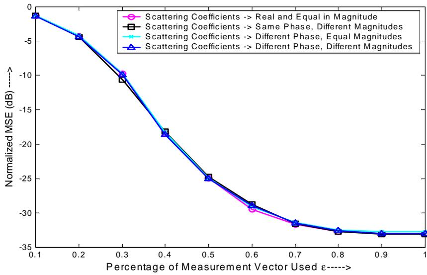
Figure 5.5 Normalized MSE (dB) vs. the fraction of measurement data processed for random scattering coefficients
