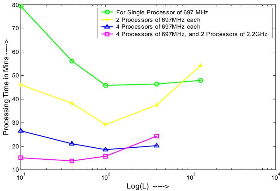
**Figure 6.2 Processing time versus L for different number of parallel processors used**
