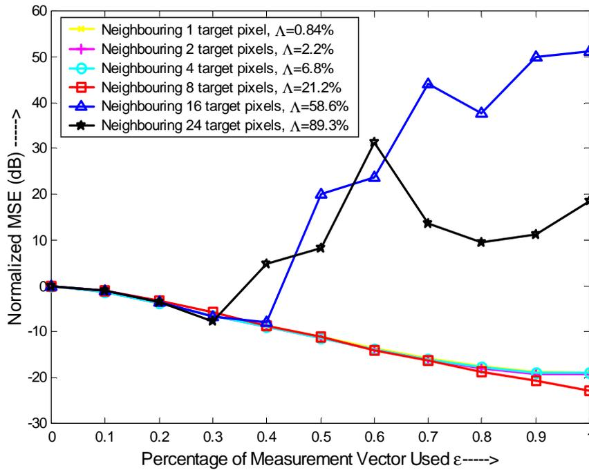
**Figure 5.19 Normalized MSE versus the fraction of measurement used for different correlation characteristics**
