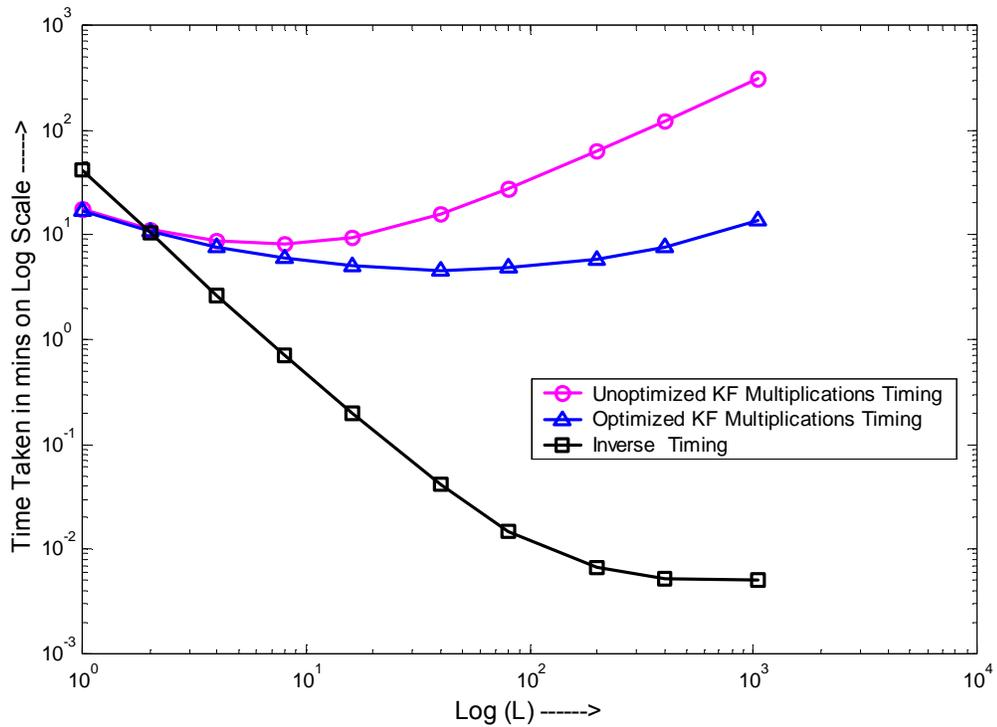
**Figure 5.2 Processing time taken versus  $L$  for KF Implementation in Matlab**
