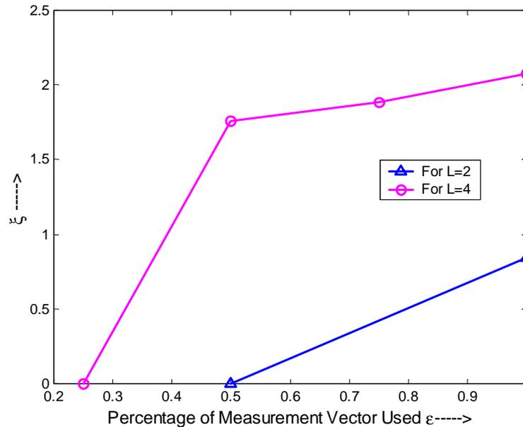
**Figure 5.11**  $\times$  The normalized Variation between  $G_u$  and  $G$  versus fraction of measurement vector processed for  $L=2$  and  $L=4$
