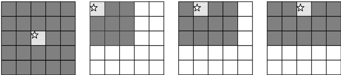
**Figure 5.17 Shows the target pixels (dark shade) supposed to be highly correlated to the concerned target pixel ('star') located at different parts of the region concerned**
