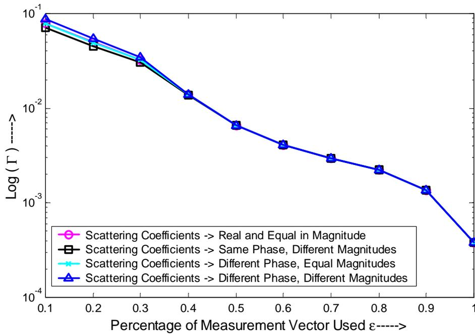
**Figure 5.7 RMS value of elements of Kalman Gain Matrix vs. the fraction of measurement data processed for random scattering coefficients**
