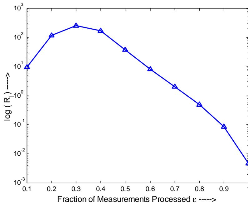
**Figure 4.4 The ratio between the absolute mean of the diagonal elements of  $\mathbf{b}$  to that of the variance of noise vs. the fraction of measurements processed  $\epsilon$**
