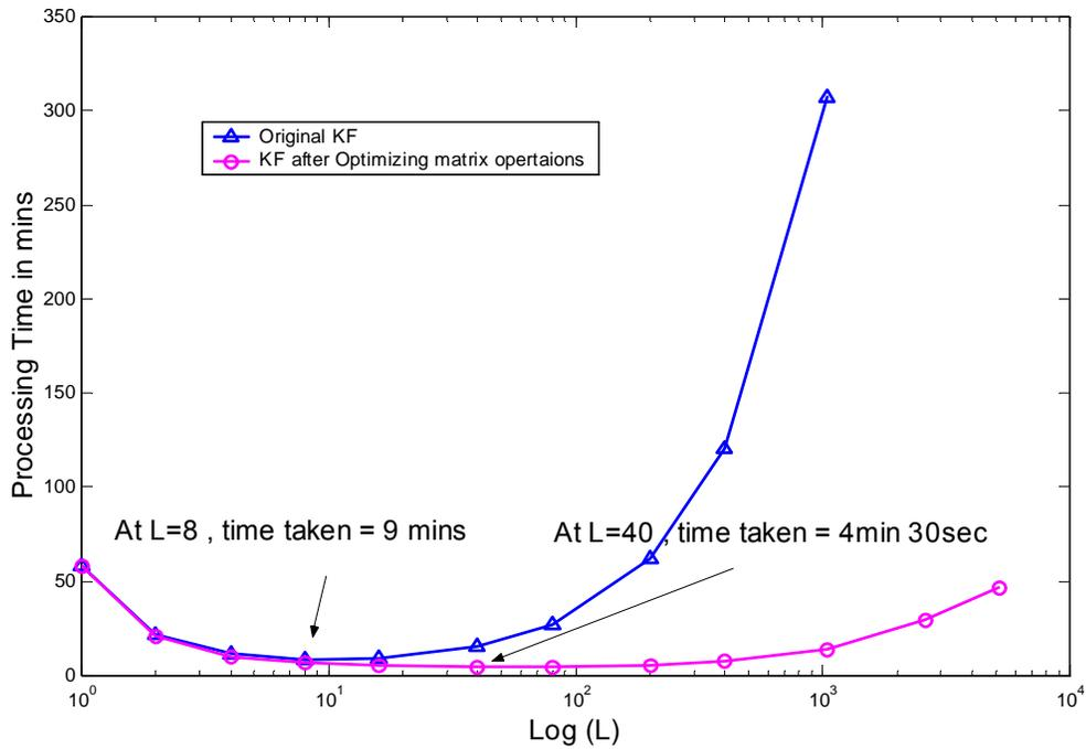
**Figure 5.3 Total Processing time taken versus  $L$  for KF Implementation in Matlab**
