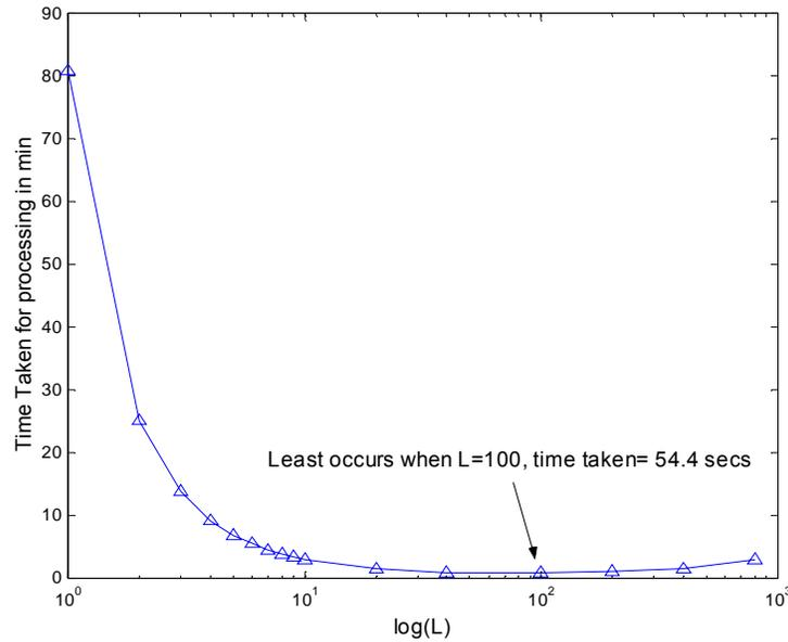
**Figure 5.12 Processing time taken versus  $L$  for a case in which only the diagonal elements are considered in the error correlation matrix  $\mathbf{K}_g$**
