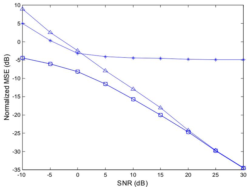
**Figure 3.8 Matched, ML, MMSE, and Kalman Filters performance versus Input SNR for 13 receiver sparse random array**
