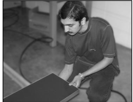
Graduate student Karthik Ramakrishnan adjusts an antenna used in RFID testing. The antenna is connected to an RFID reader that sends out electromagnetic waves, which an RFID tag's antenna is tuned to receive.
