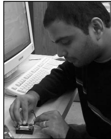
Ph.D. student Pradeepkumar Mani programs tiny devices called “motes” for the SensorNet project. Sensors will be attached to the programmed motes. The mote will then collect data from the sensor and transmit the data to a collection point.
