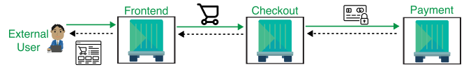
Figure 1: Sample Microservice System – Within the microservice eCommerce system, each microservice interacts with one another through service proxies that handle network communication and security logic.
