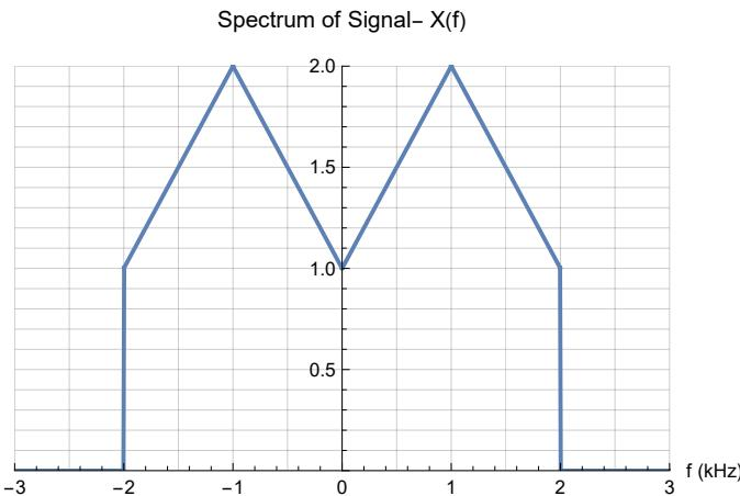
**13.** The signal  $x(t)$  is sampled at 5000 samples/sec to form  $x_s(t)$ . Plot the spectrum of  $x_s(t)$ .
