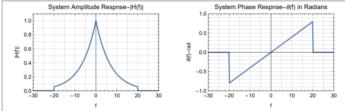
a. The signal  $x(t) = \cos(2\pi 2.5t) + \cos(2\pi 12.5t)$  is the input to the system with the frequency response  $H(f)$  given above. Find the system output,  $y(t)$ .
