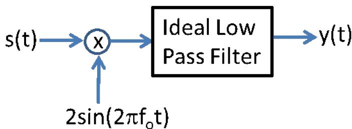
b. Find the output  $y(t)$  in terms of  $x(t)$  and  $z(t)$  of the system above. The bandwidth of the ILPF is 11 kHz. [Hint: use the trigonometry identities for  $\sin^2(\theta)$  and  $\cos^2(\theta)$ ]
