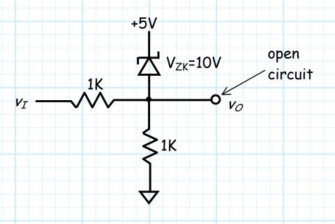
This circuit is a junction diode limiter!
