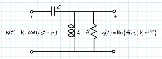
The magnitude and phase of the **output** sinusoid (expressed as **complex** value  $V_2$ ) is related to the magnitude and phase of the **input** sinusoid (expressed as **complex** value  $V_1$ ) by the system **eigen value**  $G(\omega_a)$ :
