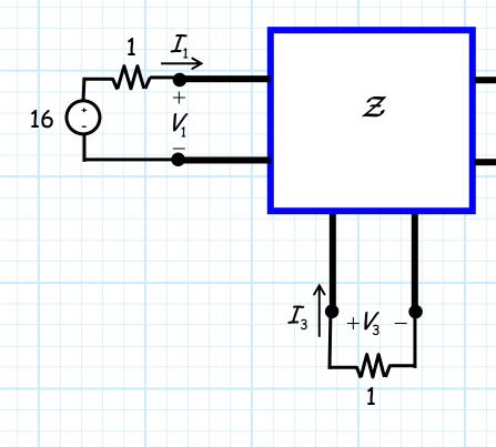
Where the 3-port **device** is characterized by the **impedance matrix**:
