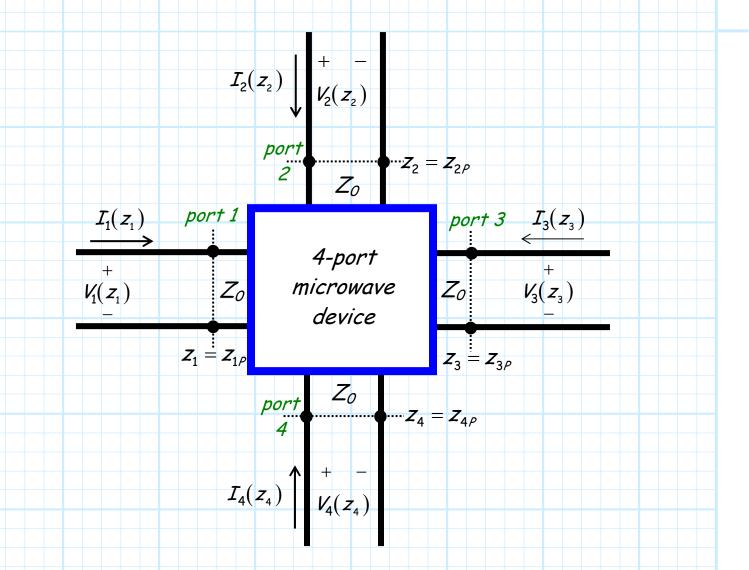
Note in this example, there are four **identical** transmission lines connected to the same "box". Inside this box there may be a very **simple** linear device/circuit, **or** it might contain a very large and **complex** linear microwave system. → Either way, the "box" can be fully characterized by its impedance matrix!
