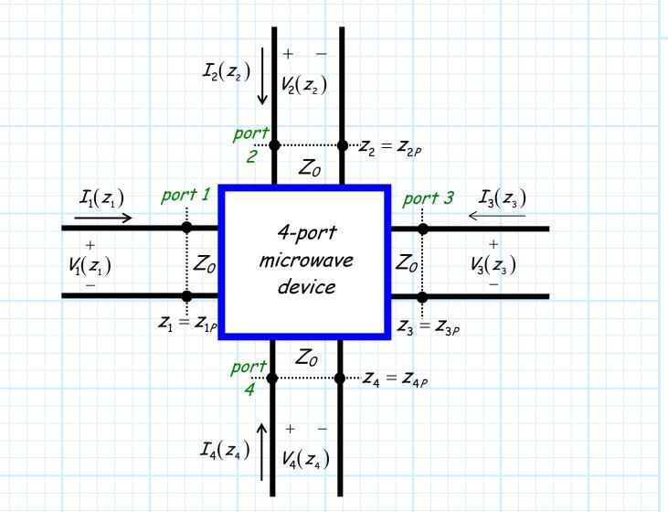
In addition to the Impedance Matrix, we can fully characterize this linear device using the Admittance Matrix.
