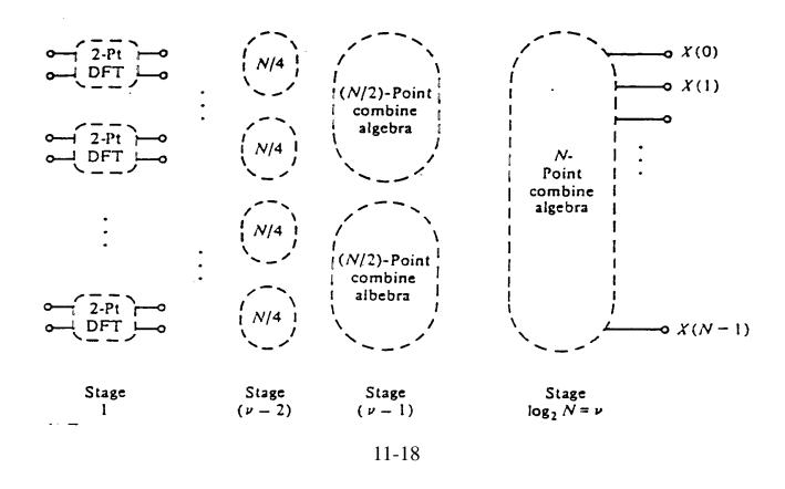
The decomposition continues until the 2-point DFT stage is reached. At this point we compute the 2-point DFT from the direct formula.
