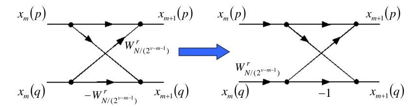
with this simplification, the number of complex multiplications required for calculating the FFT is
