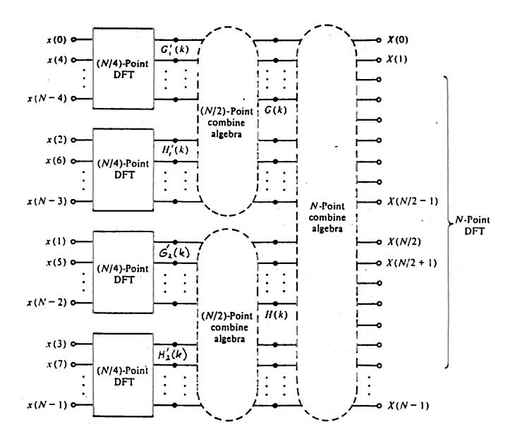
Continuing this process, each N/4 - point transform is broken into two N/8 - point DFTs, etc. Since  $N = 2^n$ , this process can be continued until there are
